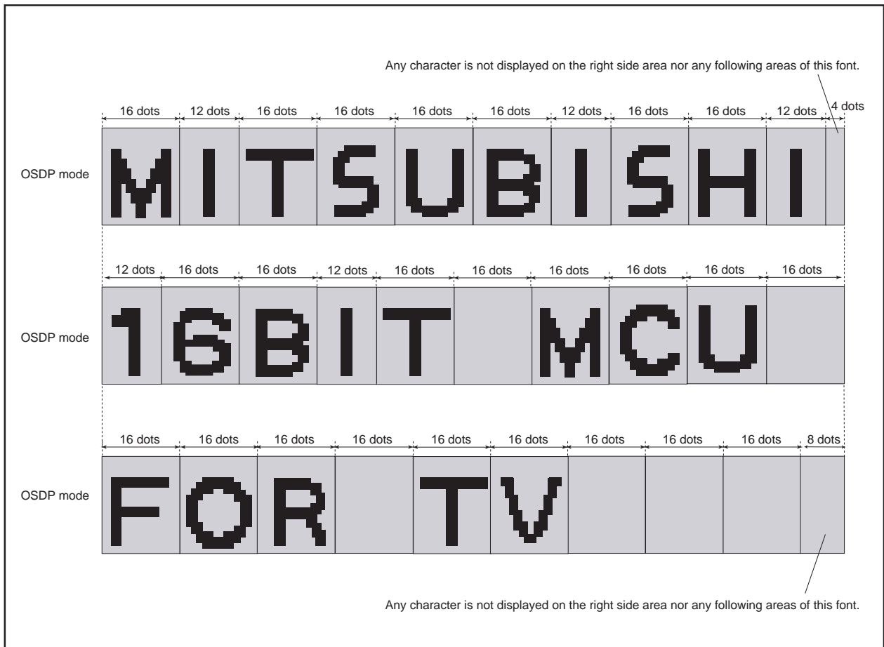
Figure 2.16.39 Display example of OSD mode block
