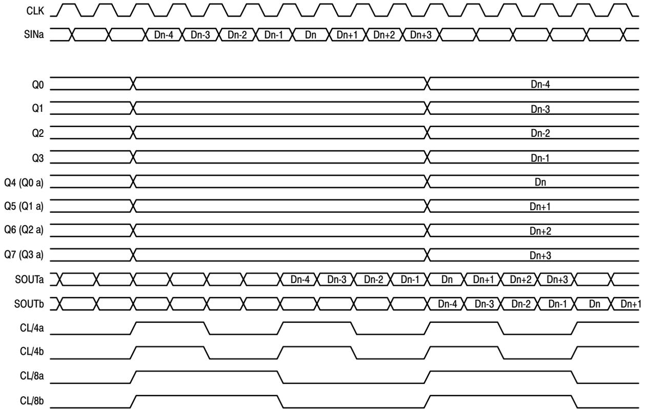
**Figure 9. Timing Diagram A. 1:8 Serial to Parallel Conversion**
