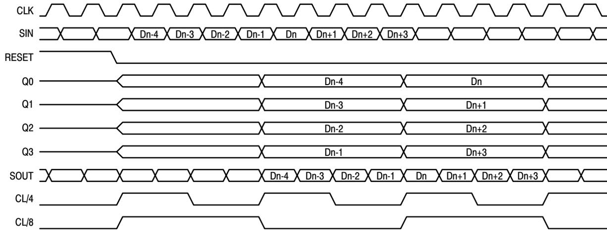
Timing Diagram A. 1:4 Serial to Parallel Conversion
