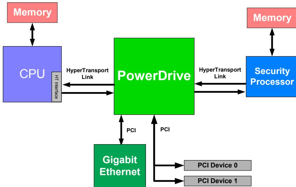
**Figure 3. Block Diagram of VPN Gateway**
