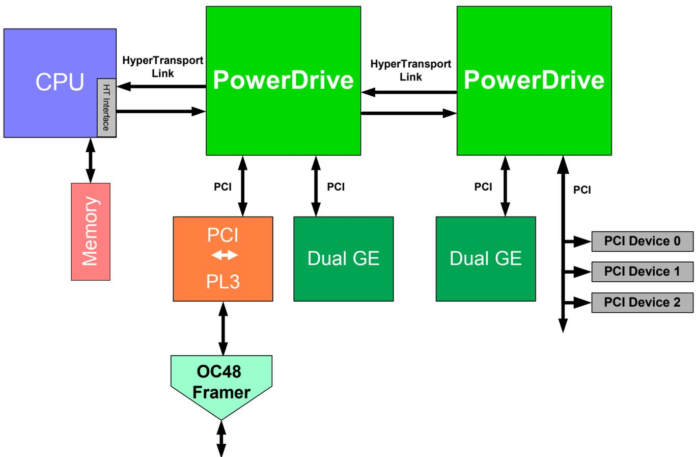
Figure 2. Block Diagram of a LAN-to-WAN Bridge/Router
