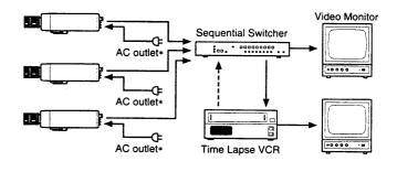
\*The SPT-M128CE operates from 220 to 240 V AC, the SPT-M124CE from 24 V AC and the SPT-M122CE from 12 V DC.
