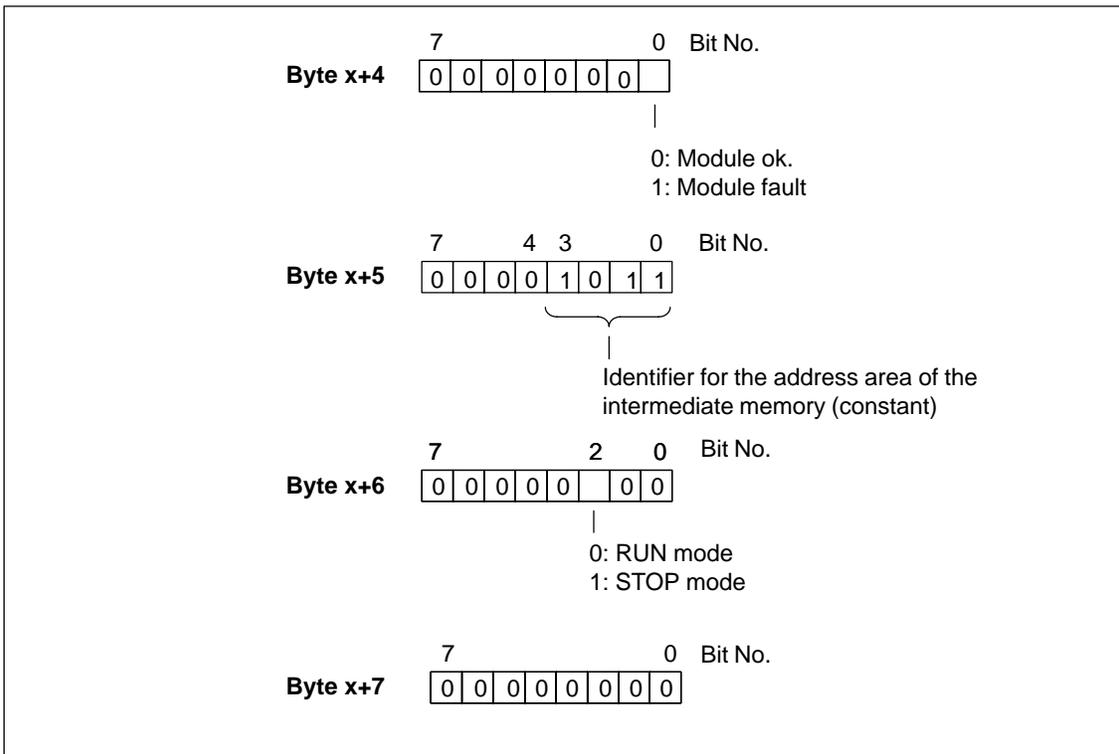
Figure 9-9 Bytes +4 to +7 for Diagnostic and Process Interrupts
