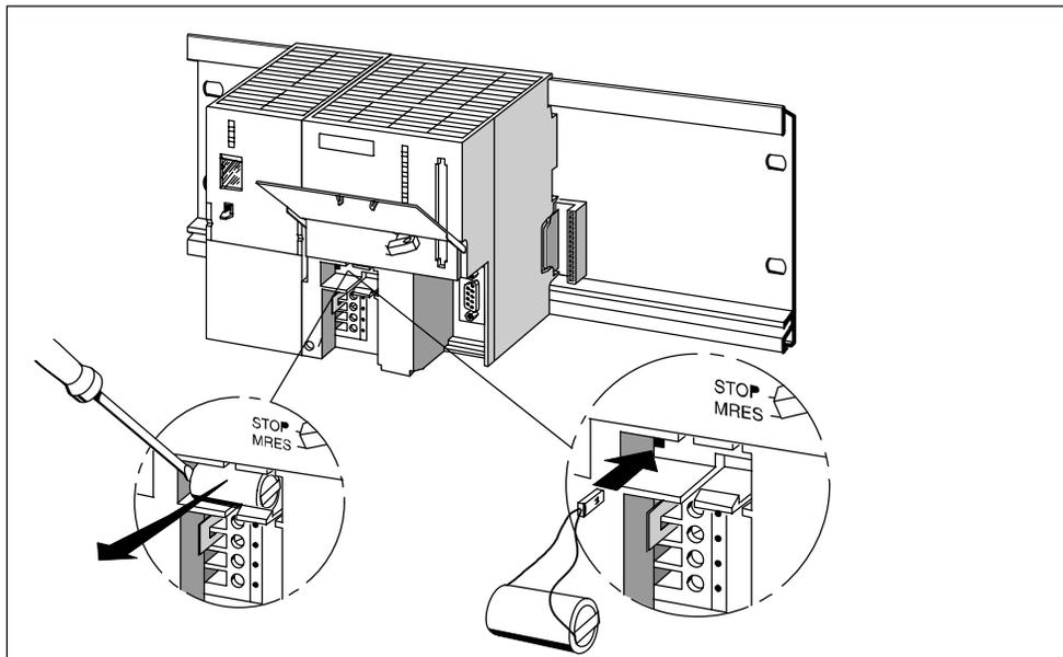
Figure 7-1 Changing the Backup Battery in the CPU 313/314
