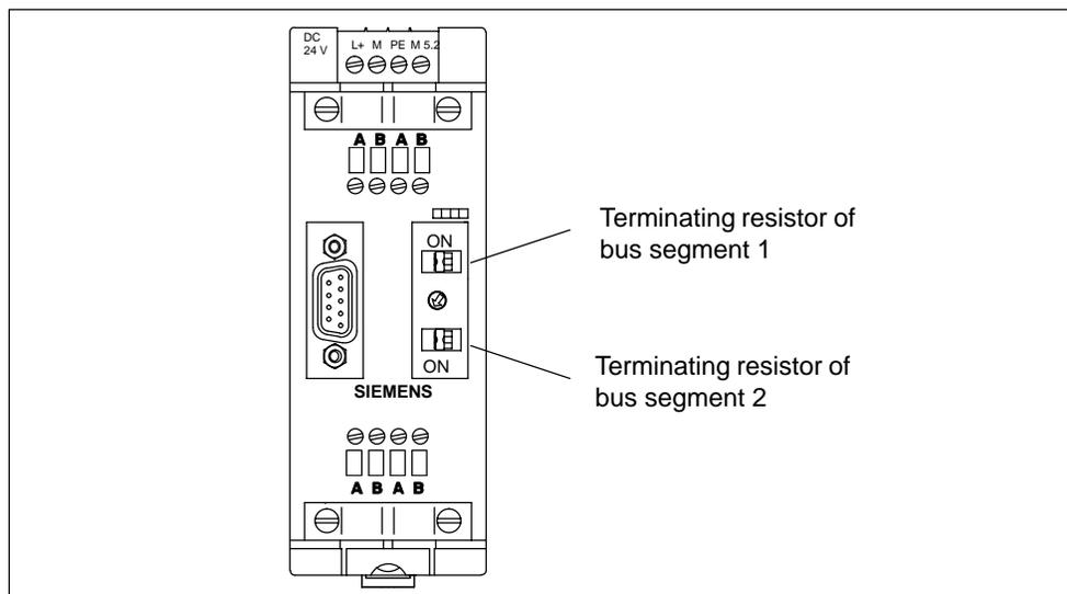
Figure 5-2 Terminating Resistor on the RS 485 Repeater
