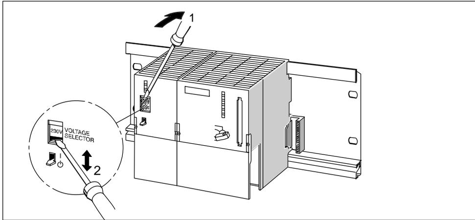
Figure 4-13 Setting the Mains Voltage for the PS 307
