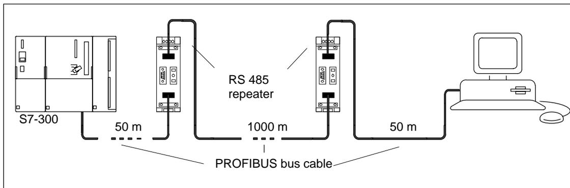
Figure 5-7 Maximum Cable Length Between Two RS 485 Repeater
