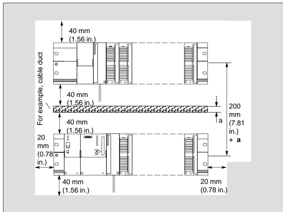
Figure 2-2 Clearance Measurements for an S7-300 Installation
