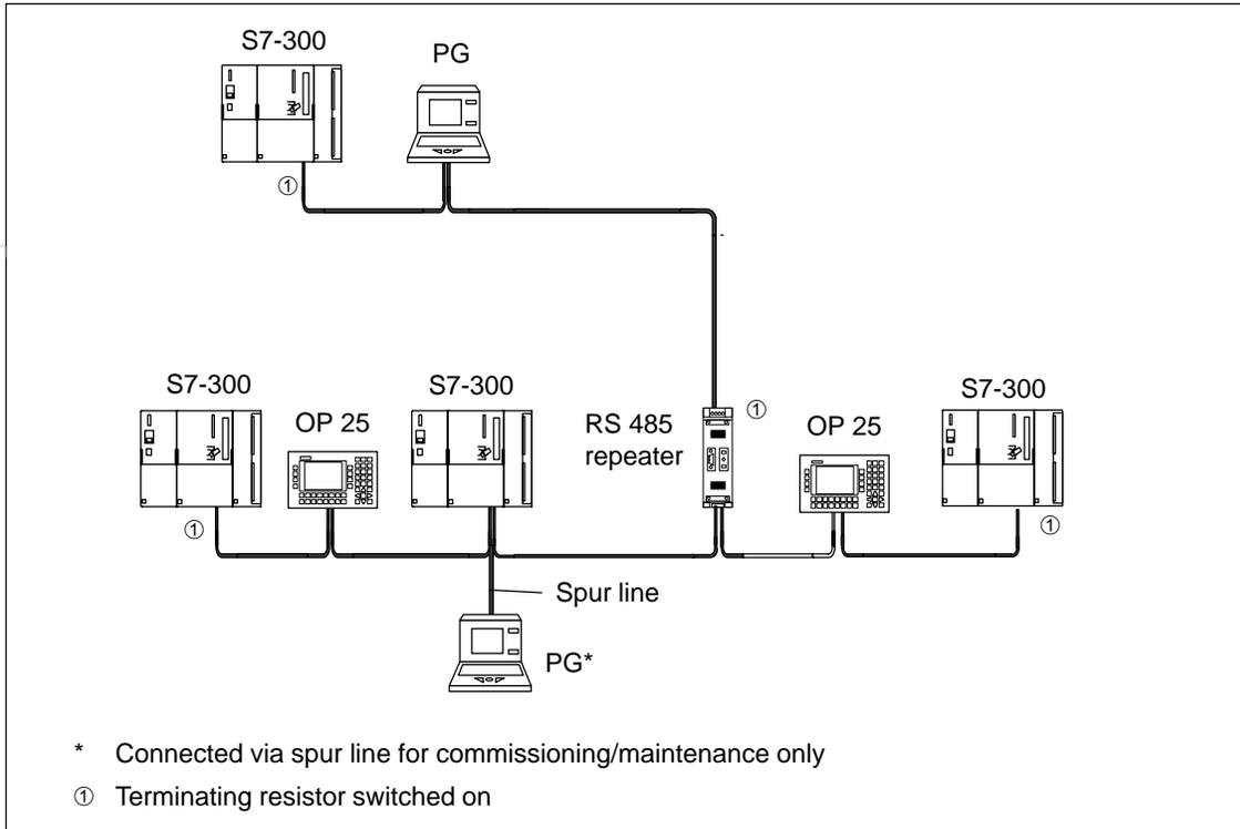
Figure 5-3 Connecting Terminating Resistors in an MPI Subnet
