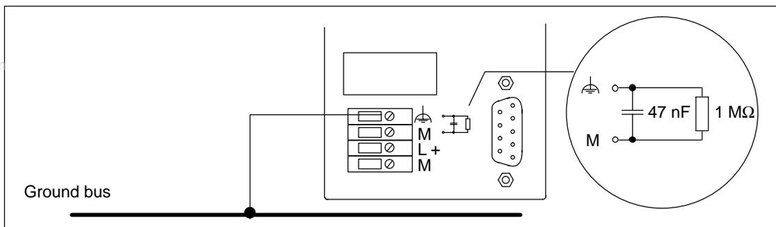
Figure 4-4 S7-300 Configuration with Ungrounded Reference Potential
