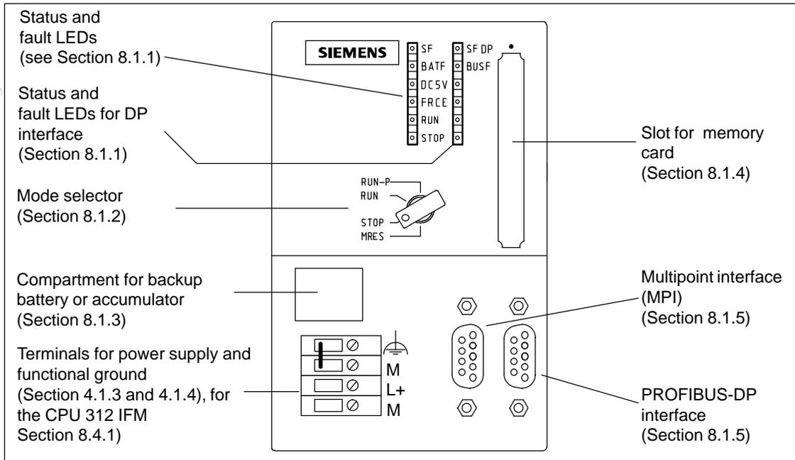
Figure 8-1 Control and Display Elements of the CPUs
