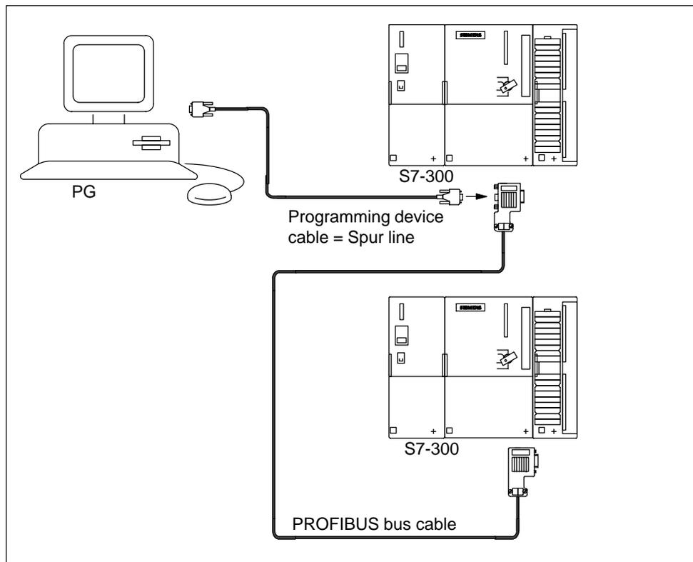
Figure 6-5 Connecting a Programming Device to a Subnet
