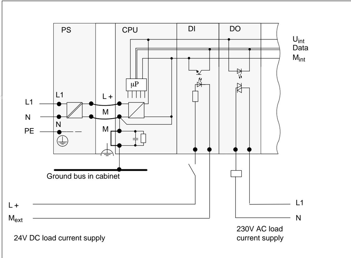
Figure 4-5 Potentials in a Configuration with Isolated Modules
