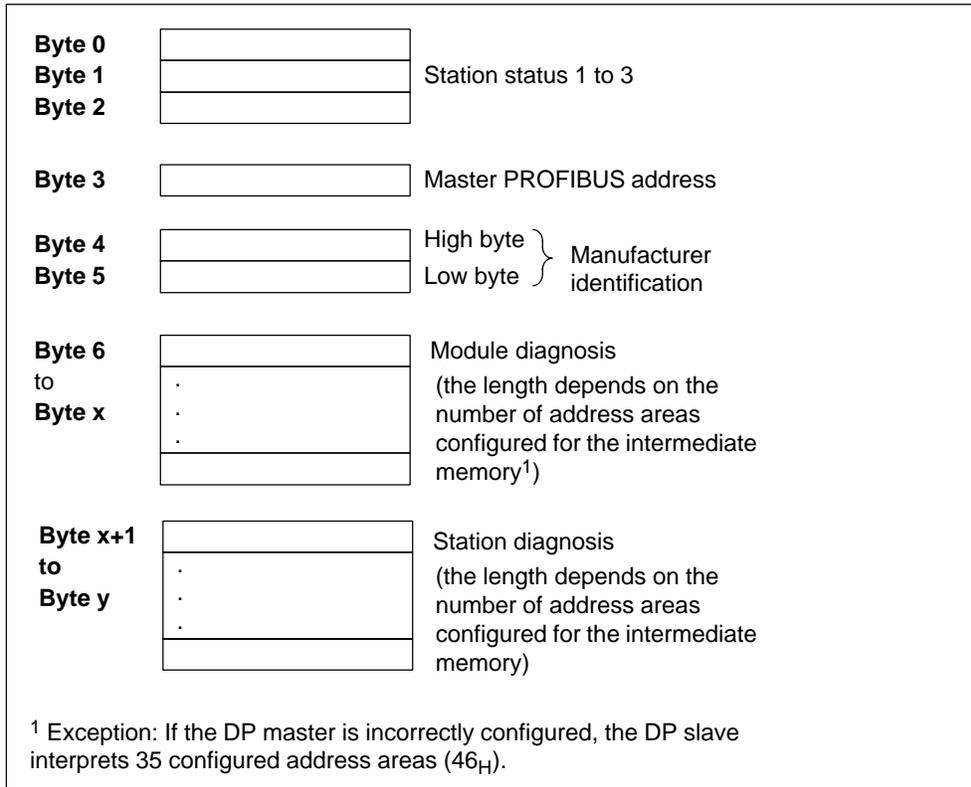
Figure 9-6 Structure of the Slave Diagnostic Data
