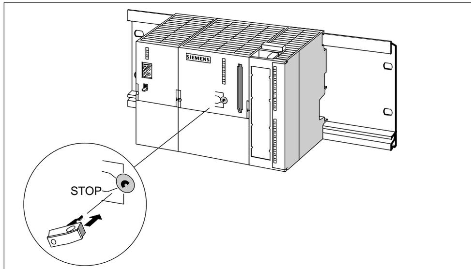
Figure 2-7 Inserting the Key in the CPU
