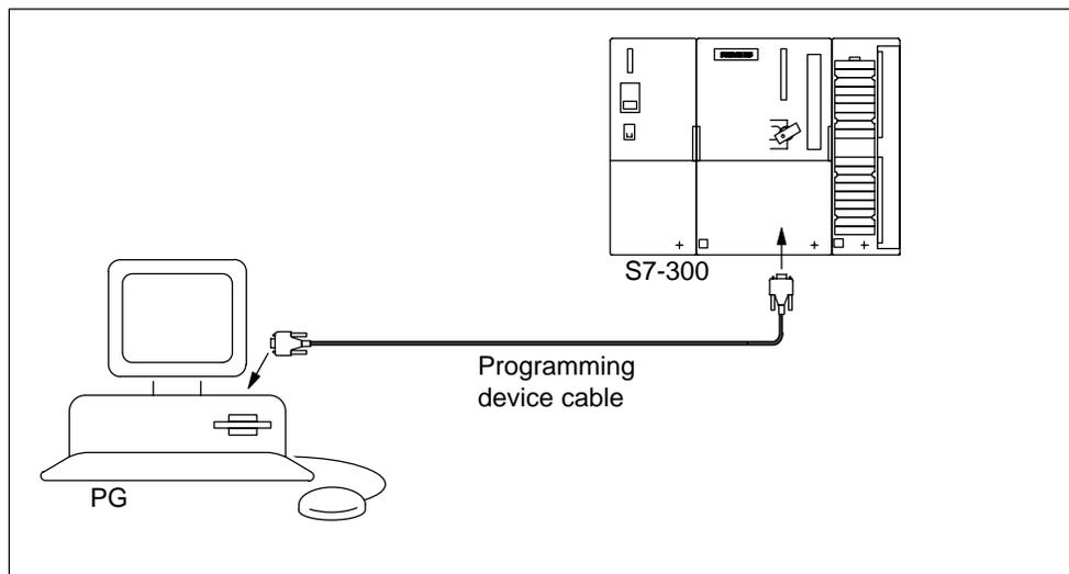
Figure 6-3 Connecting a Programming Device to an S7-300
