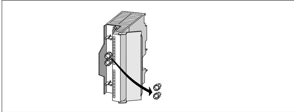
Figure 7-3 Removing the Front Connector Coding Key
