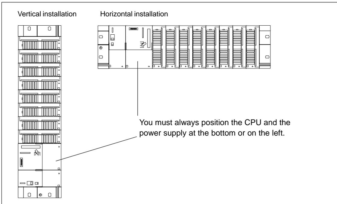
Figure 2-1 Horizontal and Vertical Installation of an S7-300
