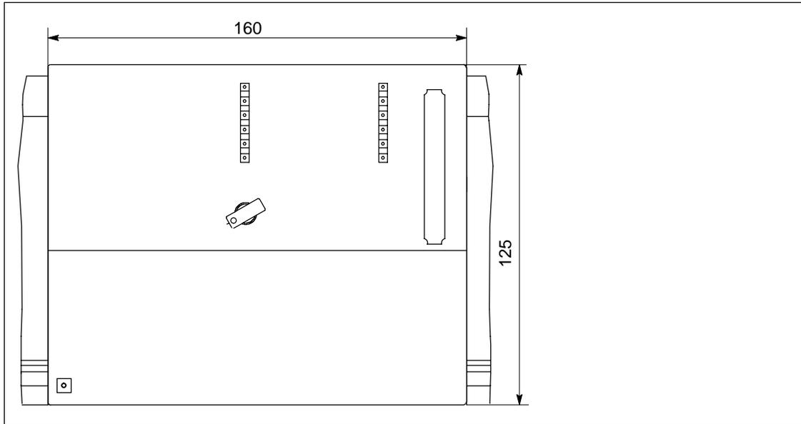
Figure E-3 Dimensioned Drawing of the CPU 318-2
