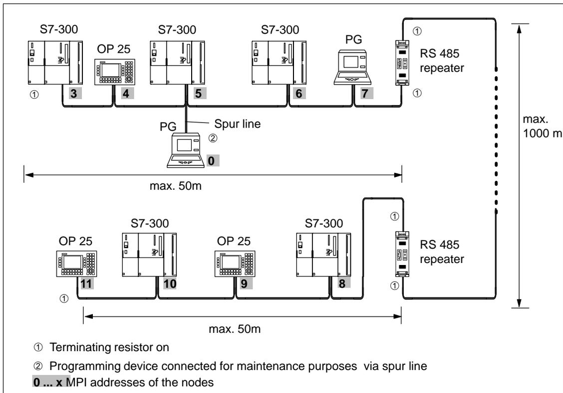
Figure 5-8 Cable Lengths in an MPI Subnet
