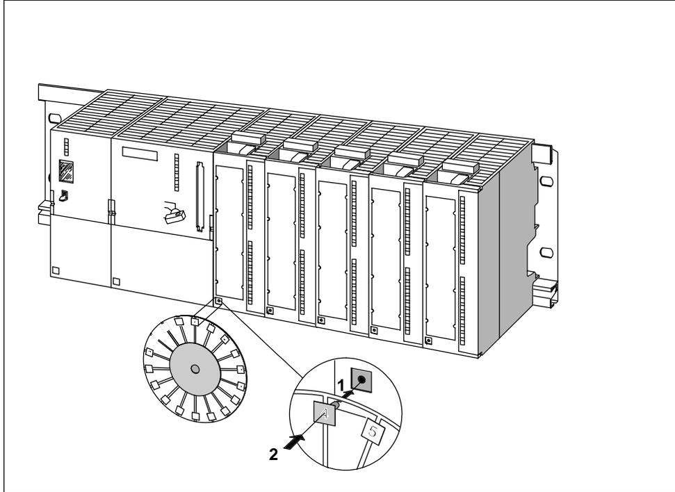
Figure 2-8 Applying Slot Numbers to the Modules
