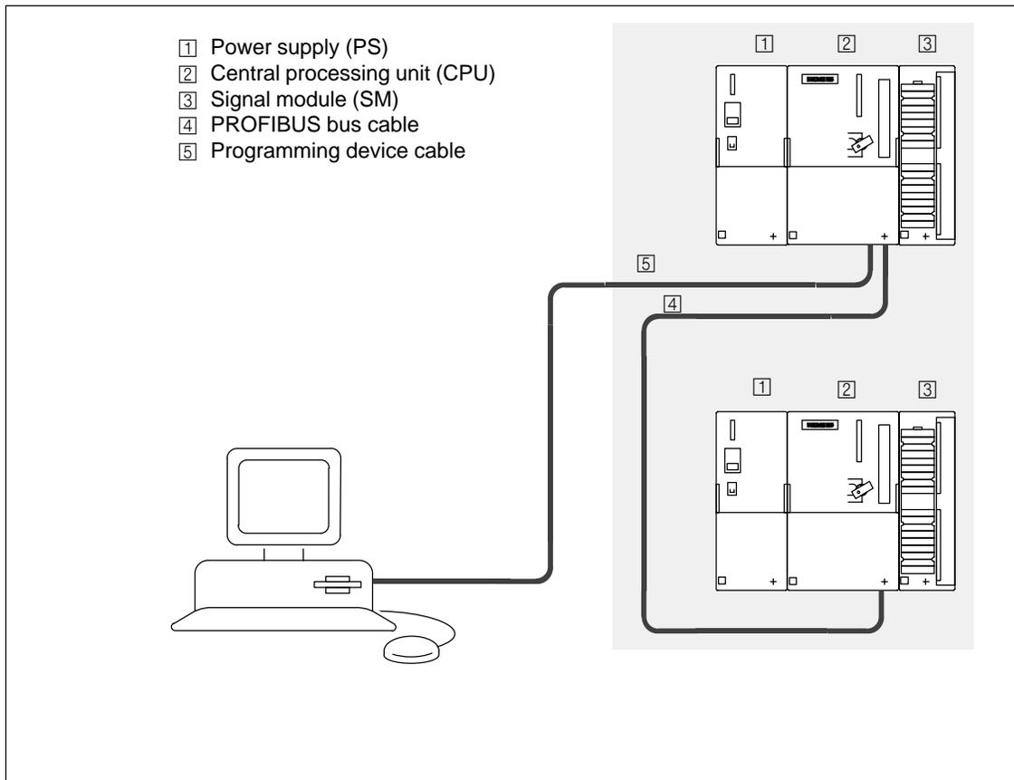
Figure 1-1 Components of an S7-300
