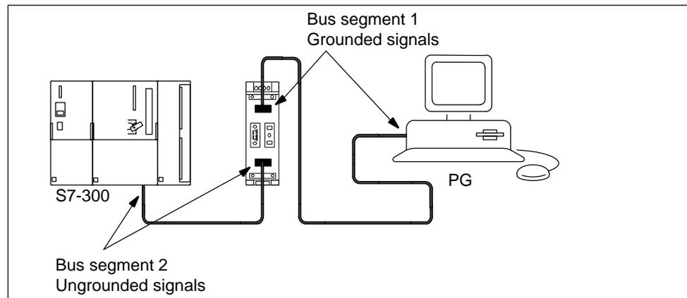
Figure 6-6 Programming Device Connected to an Ungrounded S7-300
