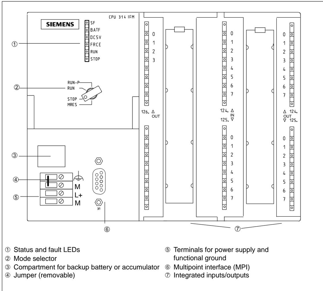
Figure 8-9 Front View of the CPU 314 IFM
