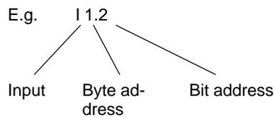
The byte address depends on the module start address.
