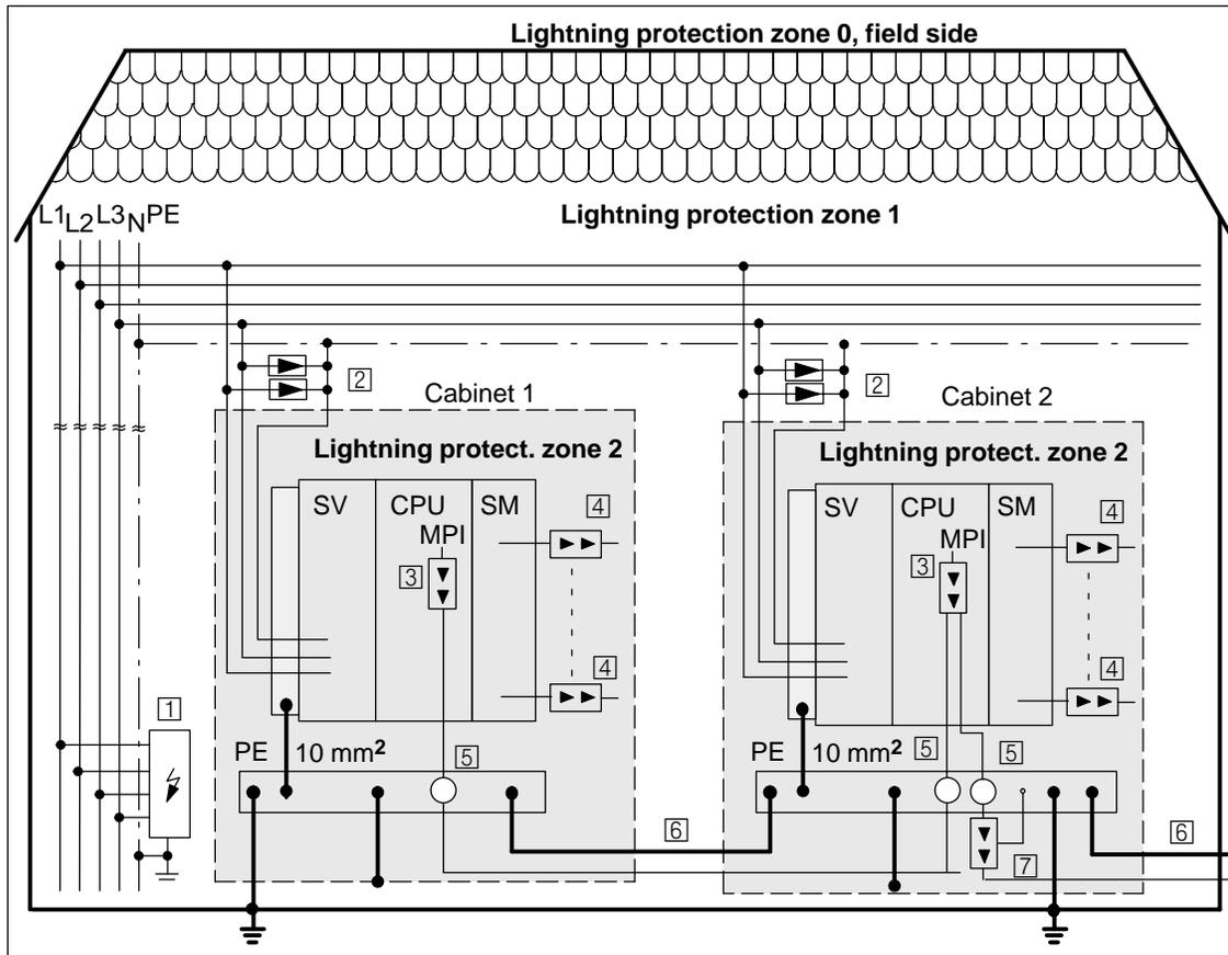
Figure 4-11 Example of the Interconnection of Networked S7-300s
