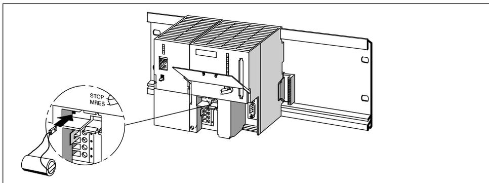
Figure 6-2 Inserting a Backup Battery in the CPUs 313/314
