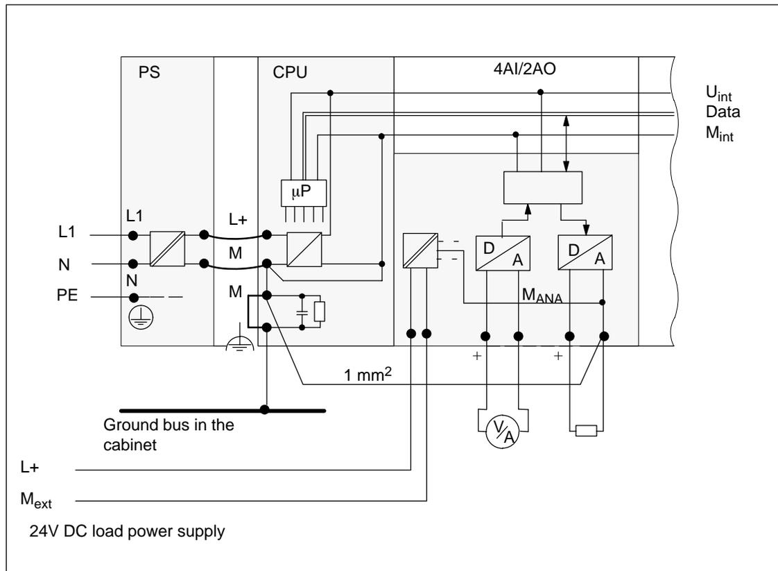
Figure 4-6 Potentials in a Configuration with the Non-Isolated SM 334 Analog Input/Output Module; AI 4/AO 2 × 8/8Bit
