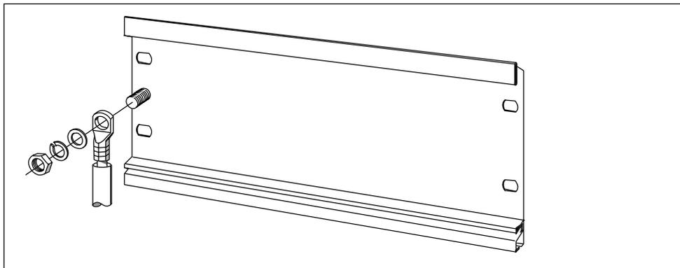
Figure 2-6 Connecting the Protective Conductor to the Rail
