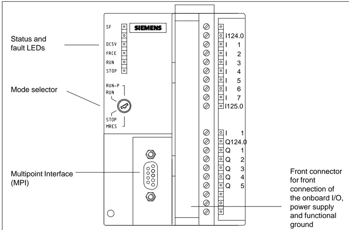
Figure 8-5 Front View of the CPU 312 IFM
