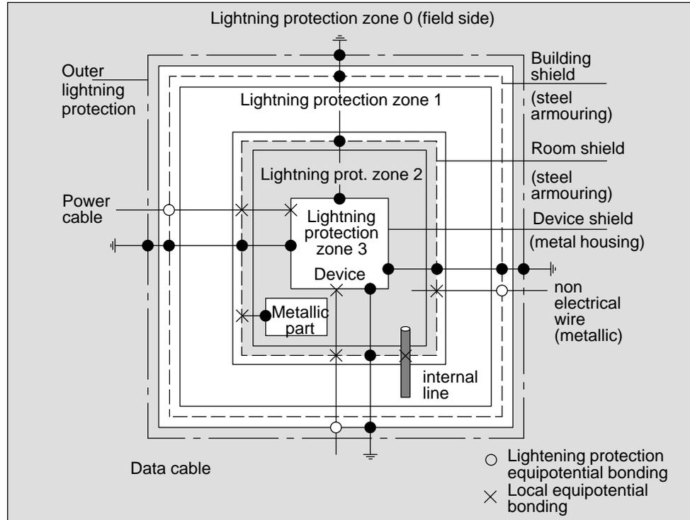
Figure 4-10 Lightning Protection Zones of a Building
