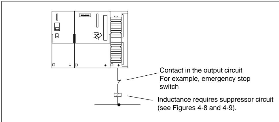
Figure 4-7 Relay Contact for Emergency Stop in the Output Circuit
