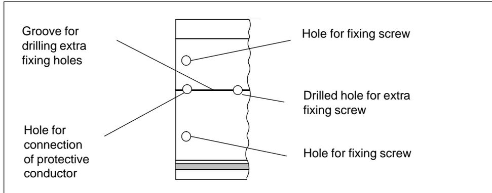
Figure 2-5 Fixing Holes of the 2 m/6.56 ft. Rail
