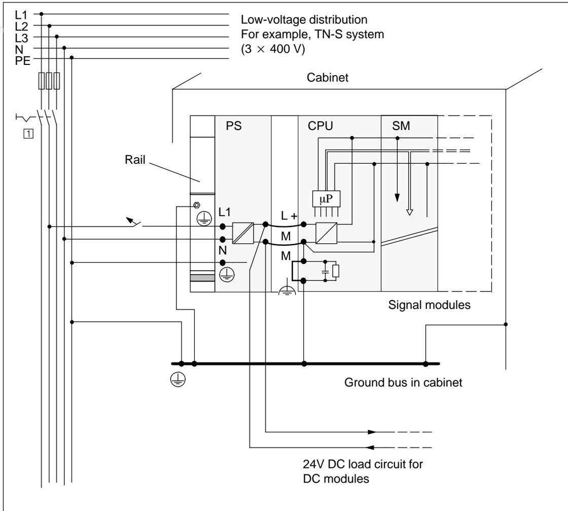
Figure 4-2 Signal Modules Powered from the PS 307
