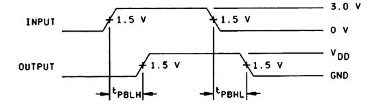
FIGURE 3. Switching waveforms and test circuit.
