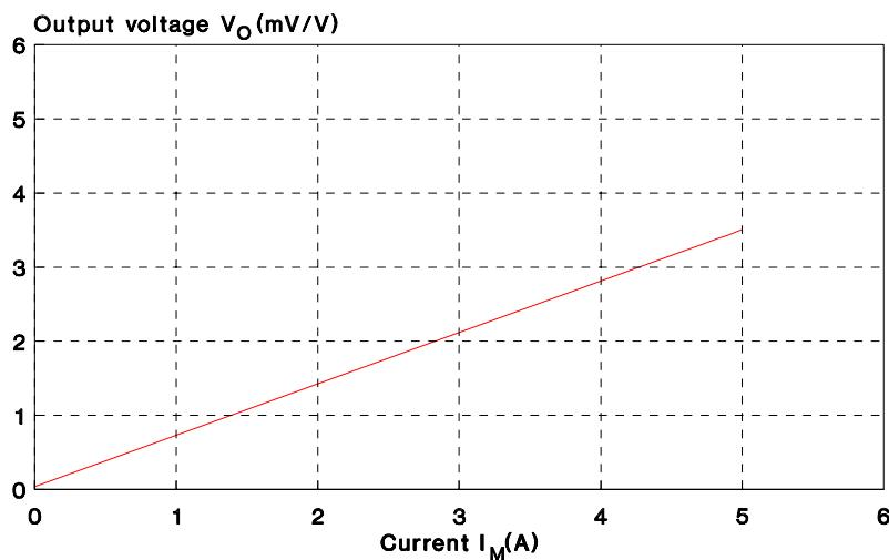
KMC 05 output voltage  $V_o$  versus current  $I_M$  for an auxiliary field  $H_x$  created by an internal magnet
