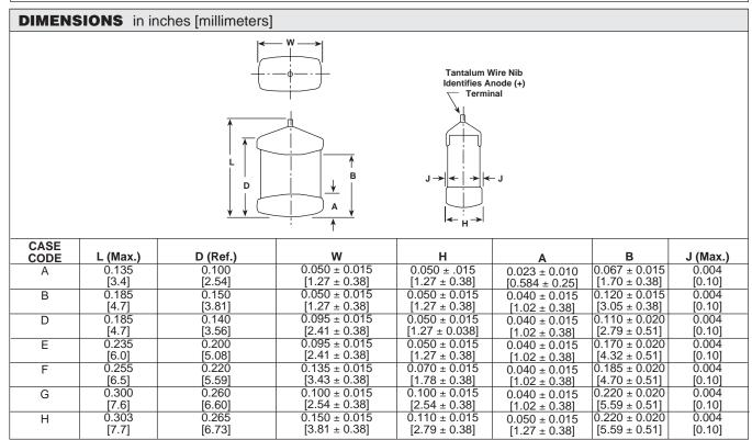
Note: The anode termination (D less B) will be a minimum of 0.010" [0.3mm]. T Case = 0.005" [0.13mm] minimum.
