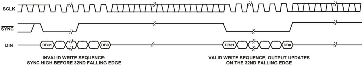
Figure 48. SYNC Interrupt Facility
