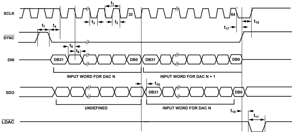
Figure 5. Daisy-Chain Timing Diagram
