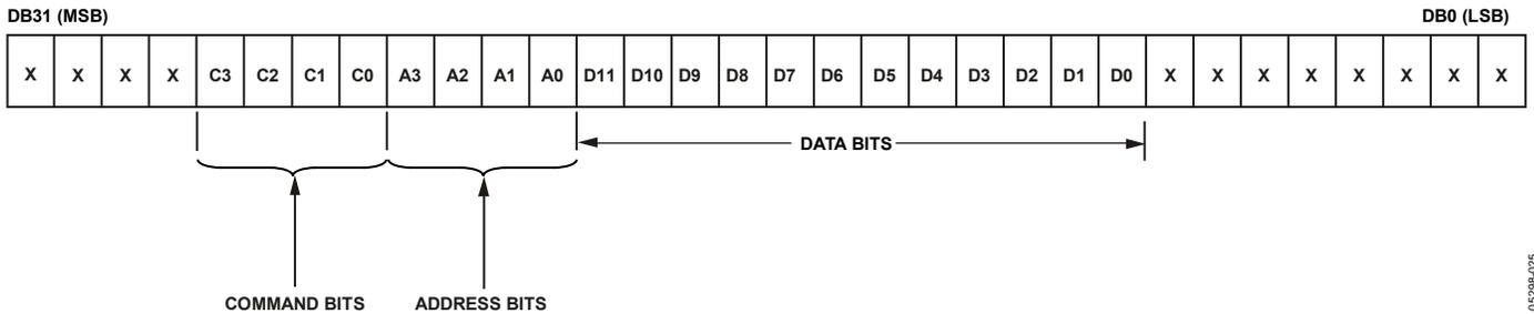
Figure 47. AD5024 Input Register Content
