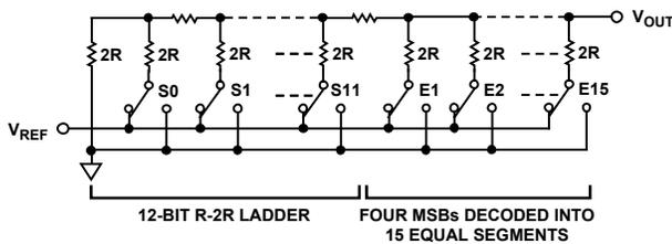
Figure 44. Dac Ladder Structure
