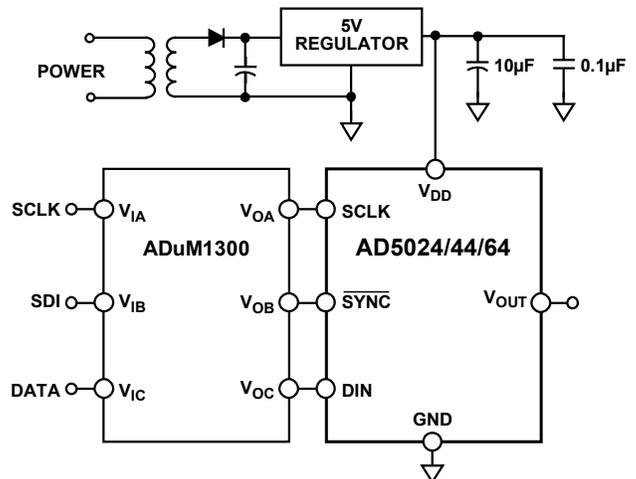
Figure 56. AD5024/44/64 with a Galvanically Isolated Interface
