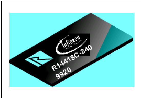
Figure 1 Direct RDRAM CSP Package
