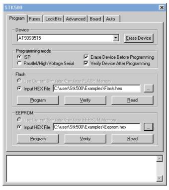
The active simulator or emulator code in AVR Studio can easily be programmed into the STK500 with a simple click of the mouse.
