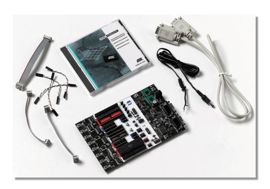
The Atmel AVR STK500 is a starter kit and development system for Atmel's AVR Flash microcontrollers. The STK500 gives designers a quick start to developing code on the AVR, combined with features for developing prototypes and testing new designs. The STK500 interfaces AVR Studio<sup>®</sup>, Atmel's Integrated Development Environment (IDE) for code writing and debugging. The STK500 starter kit includes the following:
