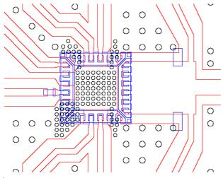
We recommend that all N/C pins be grounded and sufficient number of vias to be present under the ground plane to insure good RF and thermal grounding.
