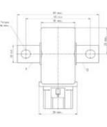
A magnetically latching power relay capable of carrying 190A at 85°C. A single short impulse to the set coil closes the relay contacts and a pulse to the reset coil opens the contacts. Designed primarily to break supply from vehicle battery in event of emergency. Typical applications are to disconnect starter motor from battery during accident, dual battery split charge applications, hydraulic pump control. IP67 sealed. Connection via amp 4 way sensor connector.
