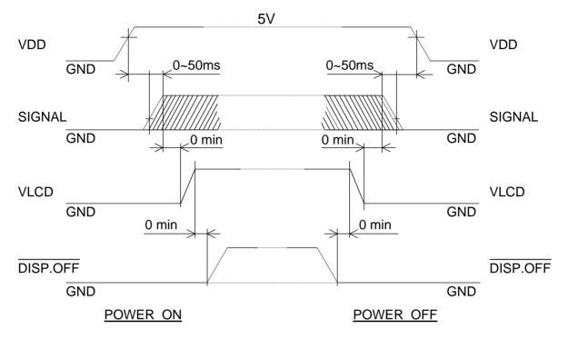
THE MISSING PIXELS MAY OCCUR WHEN THE LCM IS DRIVEN EXCEPT ABOVE POWER INTERFACE TIMING SEQUENCE.
