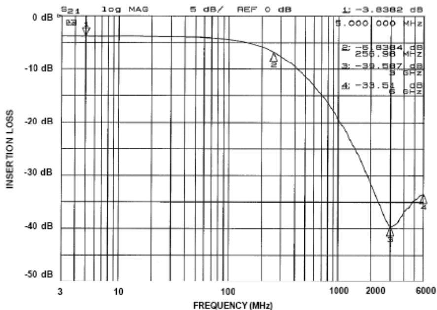
Figure 2. Insertion Loss vs. Frequency, Filter 2 (Pins 2 and 7)
