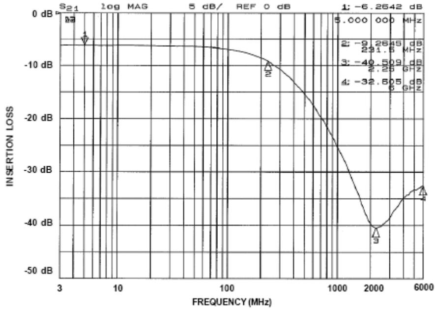
Figure 3. Insertion Loss vs. Frequency, Filter 3 (Pins 3 and 6)
