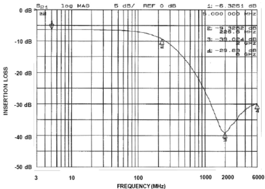
Figure 1. Insertion Loss vs. Frequency, Filter 1 (Pins 1 and 8)
