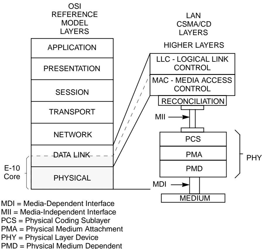
The E-10 core complies with the *Media Access Control (MAC)* sublevel within the Data Link layer of the OSI reference model and also contains a *Manchester Encoder/Decoder (ENDEC)* and *transceivers* for 10BASE-T or AUI interfaces. The ENDEC and transceivers are part of the Physical layer of the OSI model.
