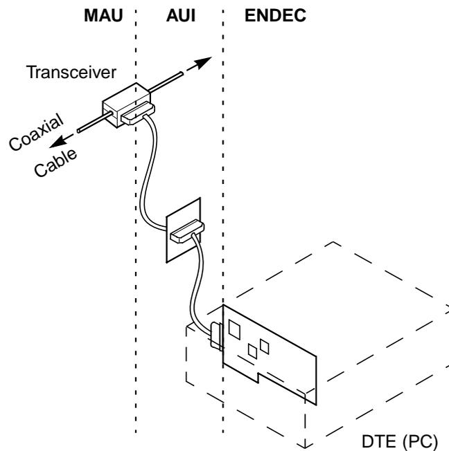
AUIs provide transmit, receive, and collision control functions. The E-10 core supports two different Attachment Unit Interface (AUI) configurations:
