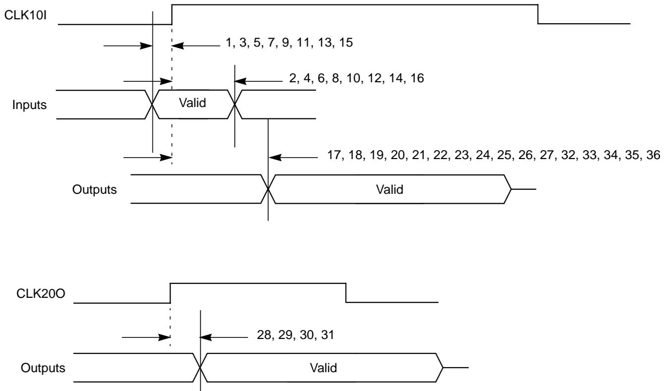
**Figure 5.2 E-10 Core Reset Timing Diagram**
