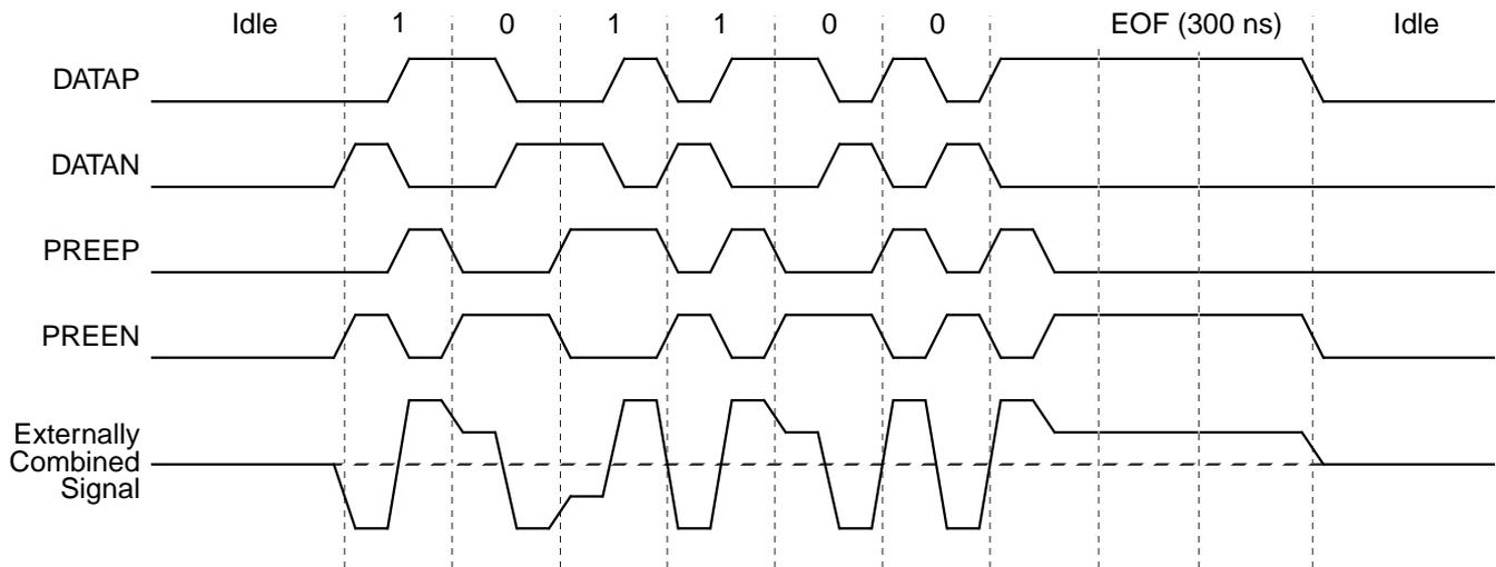
**Figure 4.9 Twisted Pair Link Integrity Pulses**
