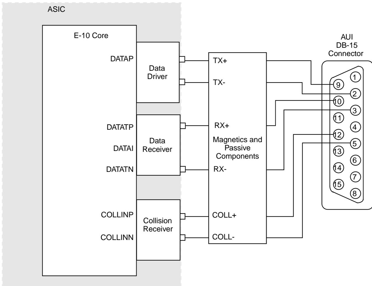
Without the integrated mixed signal I/O cores, multiple-port interfaces produce high common-mode coherent noise, which requires the use of expensive filtering to meet FCC requirements.
