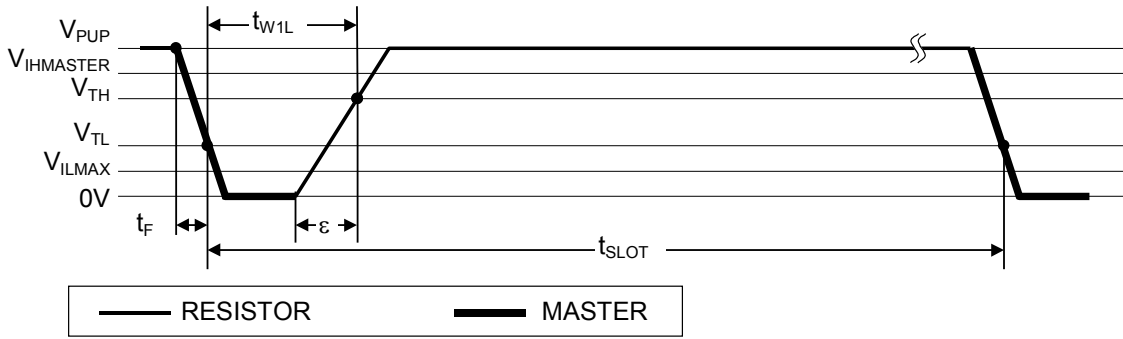
Figure 13. Read/Write Timing Diagram
