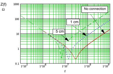
Figure 21 plots the capacitor impedance versus three different connection lengths. The resonance varies from 7 MHz to 30 MHz when the connection length varies from 0 to 5 cm.
