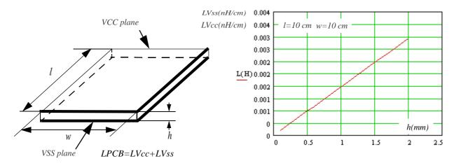
The next table shows the value of the PCB inductance for the three configurations seen above. The Vcc and Vss Power plane configuration gives the best result and a large decoupling capacitor.
