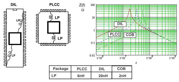
Figure 23 compares the radiated emissions between a DIL and PLCC package. Emissions can be reduced down to 7dB in the range 0.15 MHz to 400 MHz using a PLCC package instead of a DIL package.
