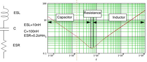
The frequency behavior depends on the type of capacitor. Table 2 gives the electrical characteristics for different capacitors.
