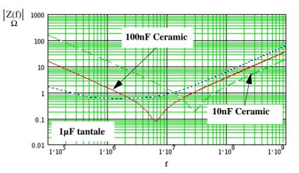
Assuming the frequency band of the noise is in the range 10MHz to 100MHz and to be compliant the network impedance has to be less than -10dBohms. Figure 20 plots the power network impedance versus the frequency and the impact of the decoupling capacitors on the impedance of the network. Five decoupling capacitors have to be added to be in the -10dBohms specification. Each capacitors is calculated to damp the pic of each frequency resonances.
