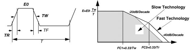
A timing analysis of the system has to be done to choose the slowest technology of the components to determine the electrical characteristics of such devices. When the maximum operation frequency limit is divided by two, EMI is reduced by 12 dB.
