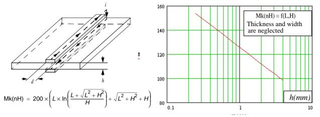
If there is no dedicated plane for the power it is recommended to maintain as close as possible the tracks to reduce the surface of loop and the parasitic inductance as shown in Figure 8.
