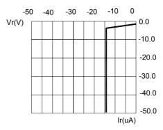
FIG.2 REVERSE CURRENT VS. REVERSE VOLTAGE.
