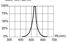
FIG.4 RELATIVE LUMINOUS INTENSITY VS. WAVELENGTH.
