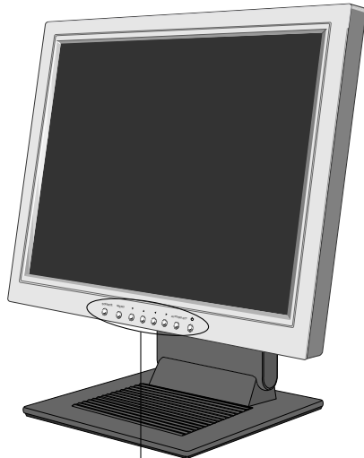
Front Control Panel
