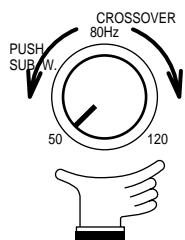
Select a crossover frequency between 50 and 120 Hz using the CROSSOVER FREQUENCY control.
