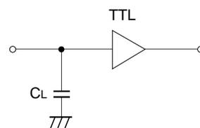
\*1 C<sub>L</sub> includes scope and jig capacitances.
