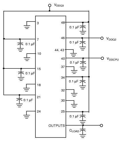
Note: All capacitors should be placed as close to each pin as possible.
