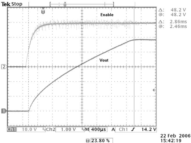
**Photo 5:** Turn On by Enable at 24 V
