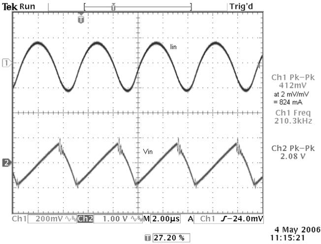
**Photo 1:** Input Ripple Voltage and Current
