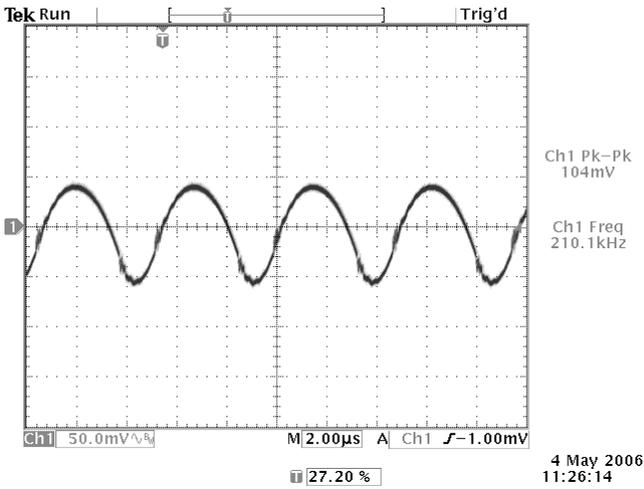
**Photo 7:** Output Ripple and Noise (20 MHz BW)
