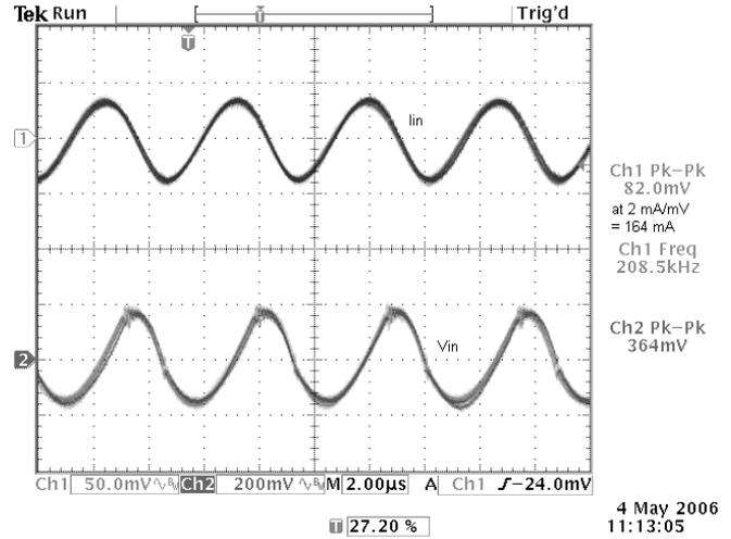
**Photo 2:** Input Ripple Voltage and Current
