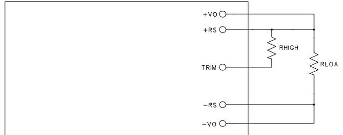
NOTE 1: CONNECT TRIM RESISTOR AS CLOSE TO CONVERTER PINS AS POSSIBLE
