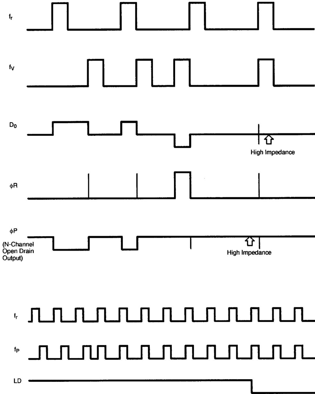
**Note:** LD is set at High level when  $f_r \neq f_v$  (unlock condition).
