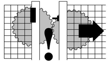
(d1) Check the machine is isolated and stopped whenever the interlocked guard door is open.
