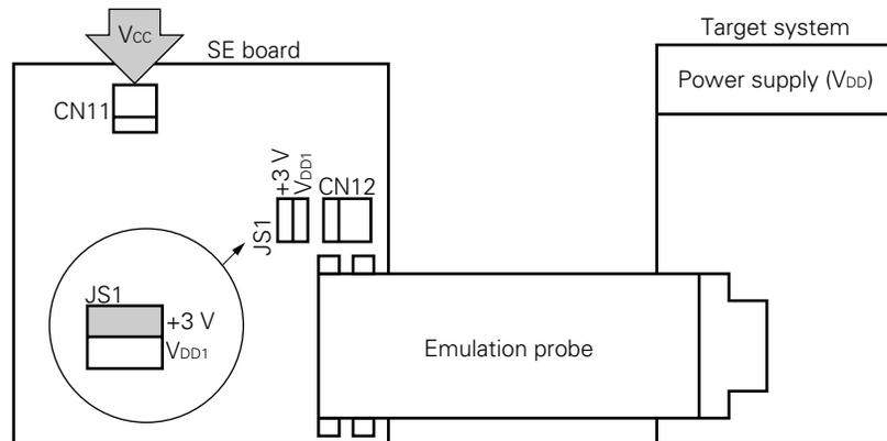
**(b) To use SE board alone with  $V_{DD} \neq +3\text{ V}$ ,  $V_{CC} = +5\text{ V}$**
