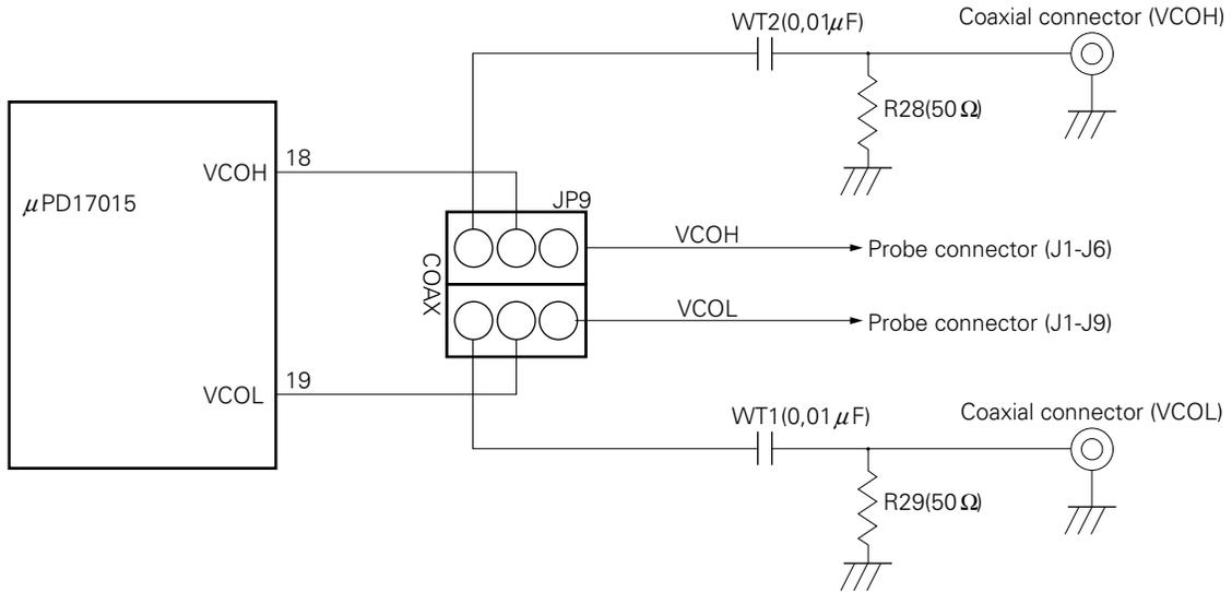
**Remark** When VCO input is from the probe, it may not be correctly input due to the influence of the wiring capacitance of the probe. It is recommended that VCOL and VCOH be input from coaxial cable to evaluate the PLL.
