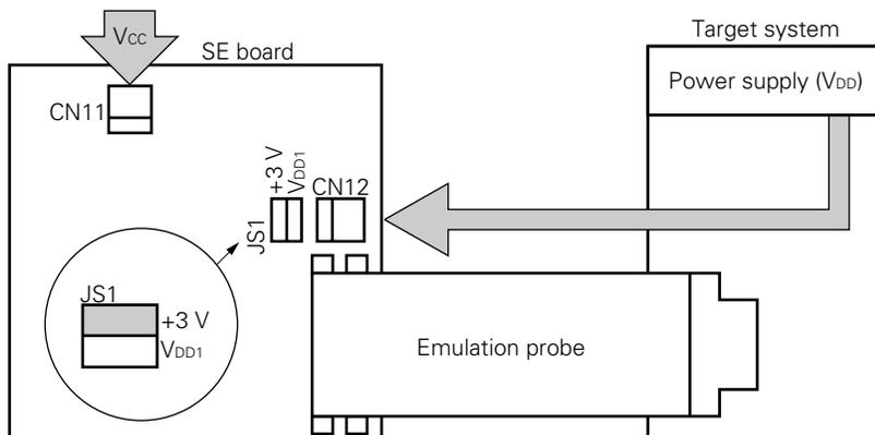
**Figure 4-6. Supplying  $V_{DD1}$  from Emulation Probe When SE Board Is Used Alone**
