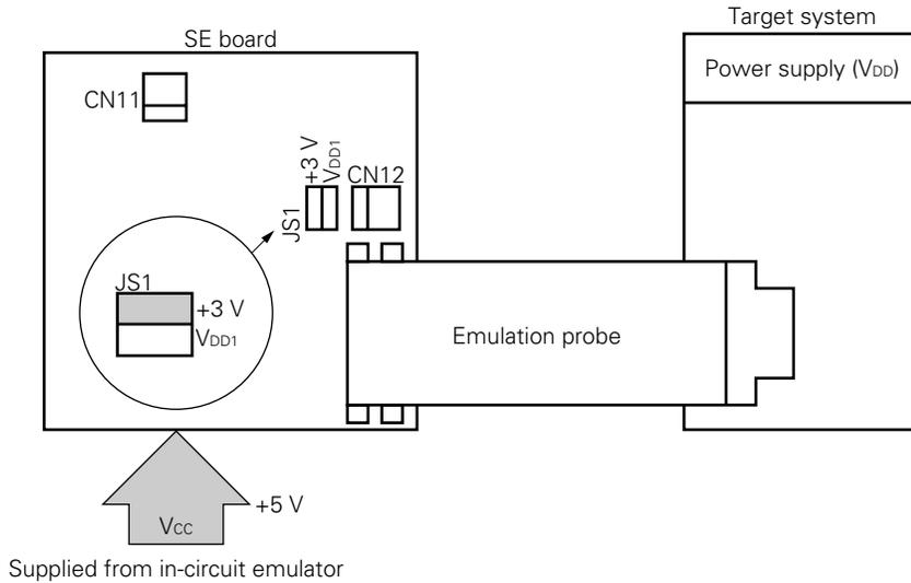
(b) To Mount SE Board in In-Circuit Emulator When  $V_{DD1} \neq +3\text{ V}$ ,  $V_{CC} = +5\text{ V}$
