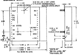
OFFSET: Connect 10K pot between P1 and P3. Wiper to P2.
