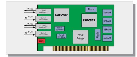
The highest density module available today with 4 channels on a small PCI short card form factor- 4.2" x 6.875".
