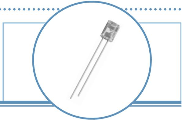
The **OVLLG8C7** is designed for superior performance in signage and lighting applications that require wide-angle, uniform light output. This device combines a high-intensity InGaN LED with a unique flat-topped T-1<sup>3</sup>/<sub>4</sub> package to provide both high brightness and a wide spatial radiation pattern.
