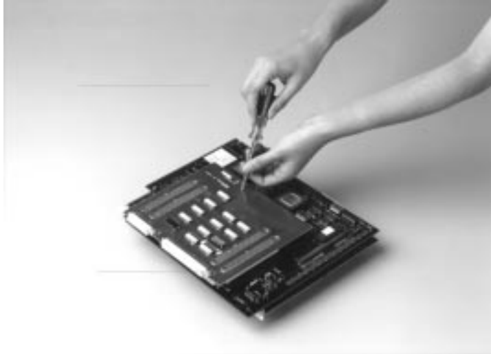
Figure 2-6. Screw Fastening of IE-75300-R-EM, IE-75000-R-BK, and Adapter Board
