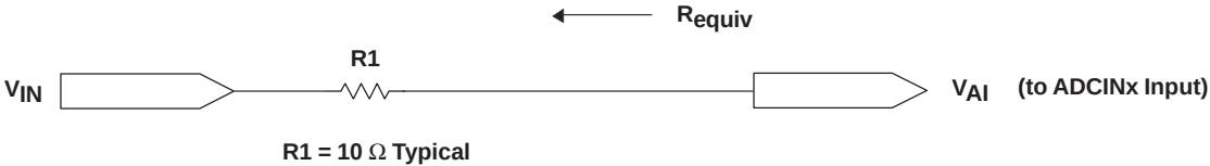
Figure 41. Typical ADC Input Pin Circuit
