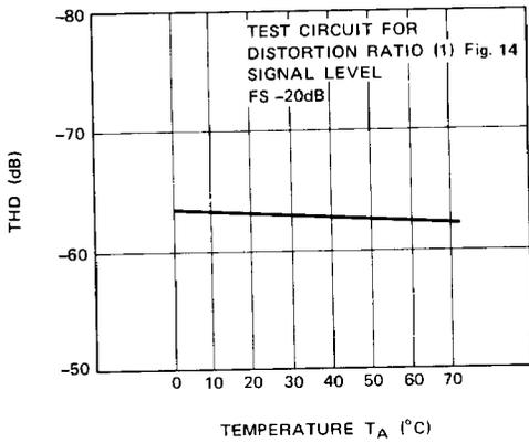
**Fig. 26 – TEMPERATURE vs. DISTORTION RATIO (D/A MODE)**
