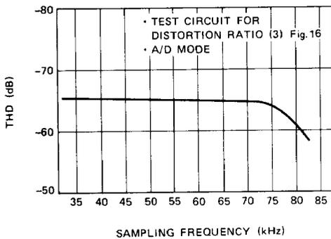
**Fig. 28 – SAMPLING FREQUENCY vs. DISTORTION RATIO**
