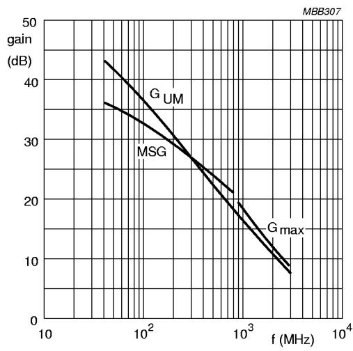
$V_{CE} = 8 \text{ V}$ ;  $I_C = 30 \text{ mA}$ .
