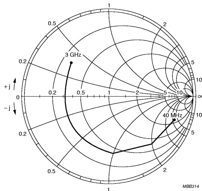
$V_{CE} = 8 \text{ V}; I_C = 15 \text{ mA}; Z_O = 50 \Omega$ .Fig.16 Common emitter input reflection coefficient ( $S_{11}$ ).
