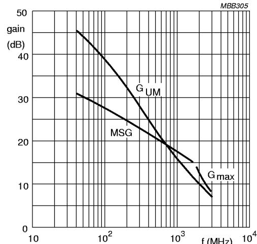
$V_{CE} = 8 \text{ V}$ ;  $I_C = 5 \text{ mA}$ .
