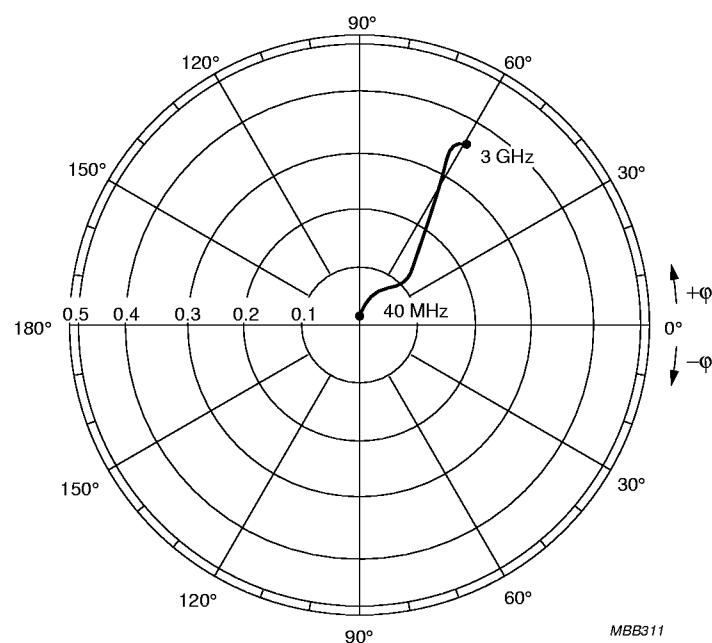
$V_{CE} = 8 \text{ V}; I_C = 15 \text{ mA}.$ Fig.19 Common emitter output reflection coefficient ( $S_{22}$ ).
