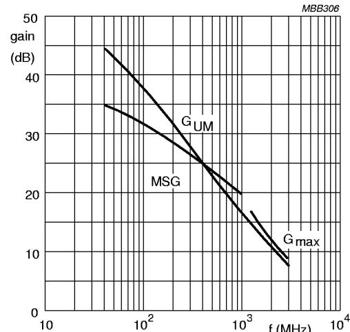
$V_{CE} = 8 \text{ V}$ ;  $I_C = 15 \text{ mA}$ .
