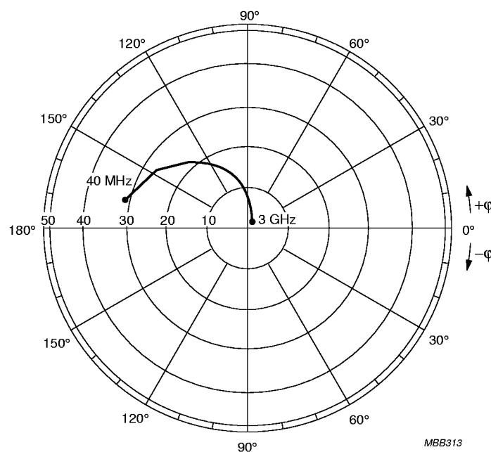
$V_{CE} = 8 \text{ V}; I_C = \text{mA}; Z_O = 50 \Omega$ .Fig.17 Common emitter forward transmission coefficient ( $S_{21}$ ).
