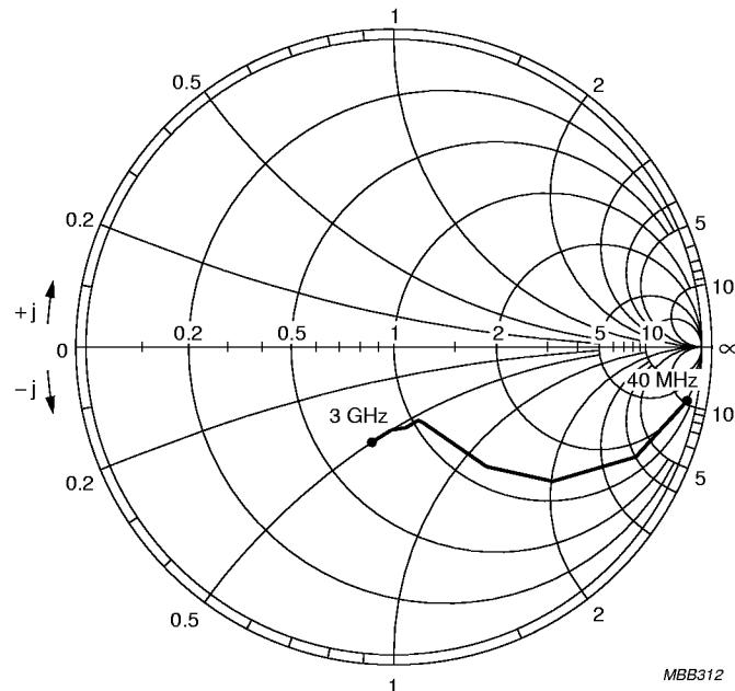
$V_{CE} = 8 \text{ V}; I_C = 15 \text{ mA}.$ Fig.18 Common emitter reverse transmission coefficient ( $S_{12}$ ).
