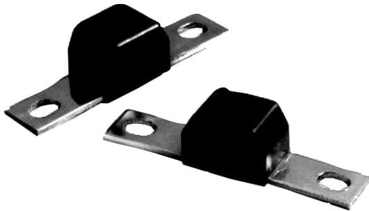
Bolt-in high current, time lag fuse. Ampere ratings from 75 to 200 Amps. IR 1,000A @ 32VDC. Ideal for use in high current heavy-duty applications such as battery and alternator cables.
