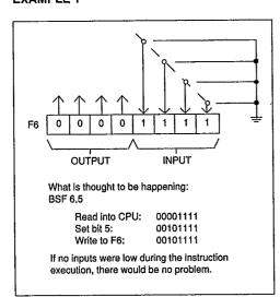
that file to be read into the CPU (MOVF, BIT SET, BIT CLEAR, and BIT TEST) is executed. Otherwise, the previous state of that pin may be read into the CPU rather than the new state. This will happen if tpd (See I/O Timing Diagram) is greater than 1/4tcy (min). When in doubt, it is better to separate these instructions with a NOP or other instruction.
