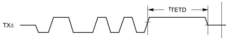
Figure 54. 10 Mbps Transmit (TX±) Timing Diagram
