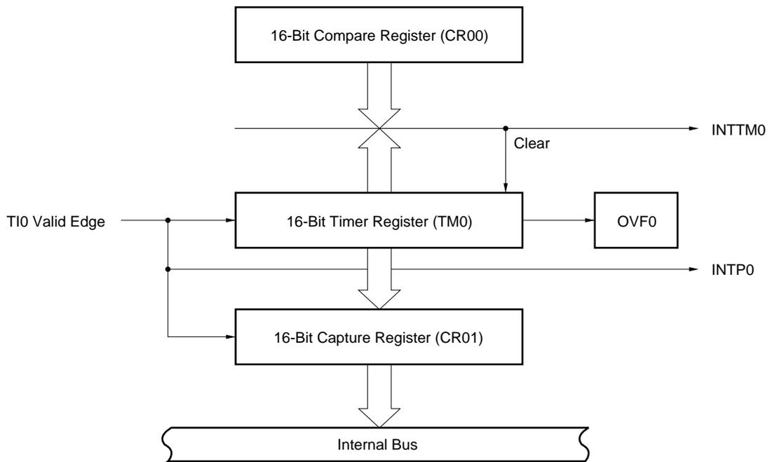
**Figure 8-18. External Event Counter Operation Timings (with Rising Edge Specified)**
