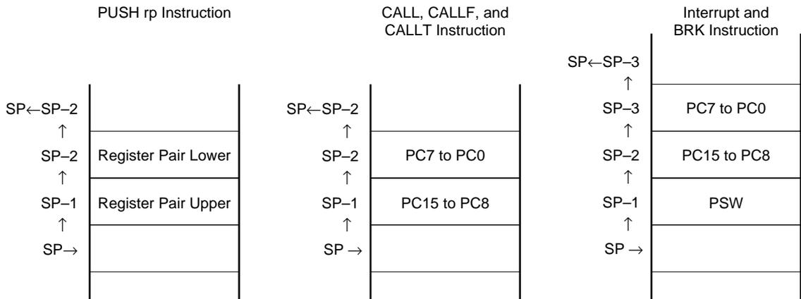
**Figure 5-10. Data to be Reset from Stack Memory**
