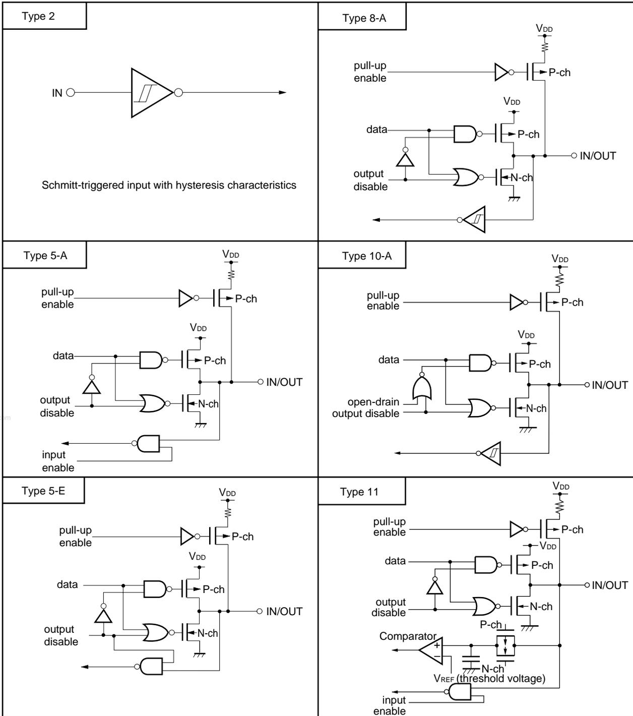
Figure 4-1. Pin Input/Output Circuit List (2/2)
