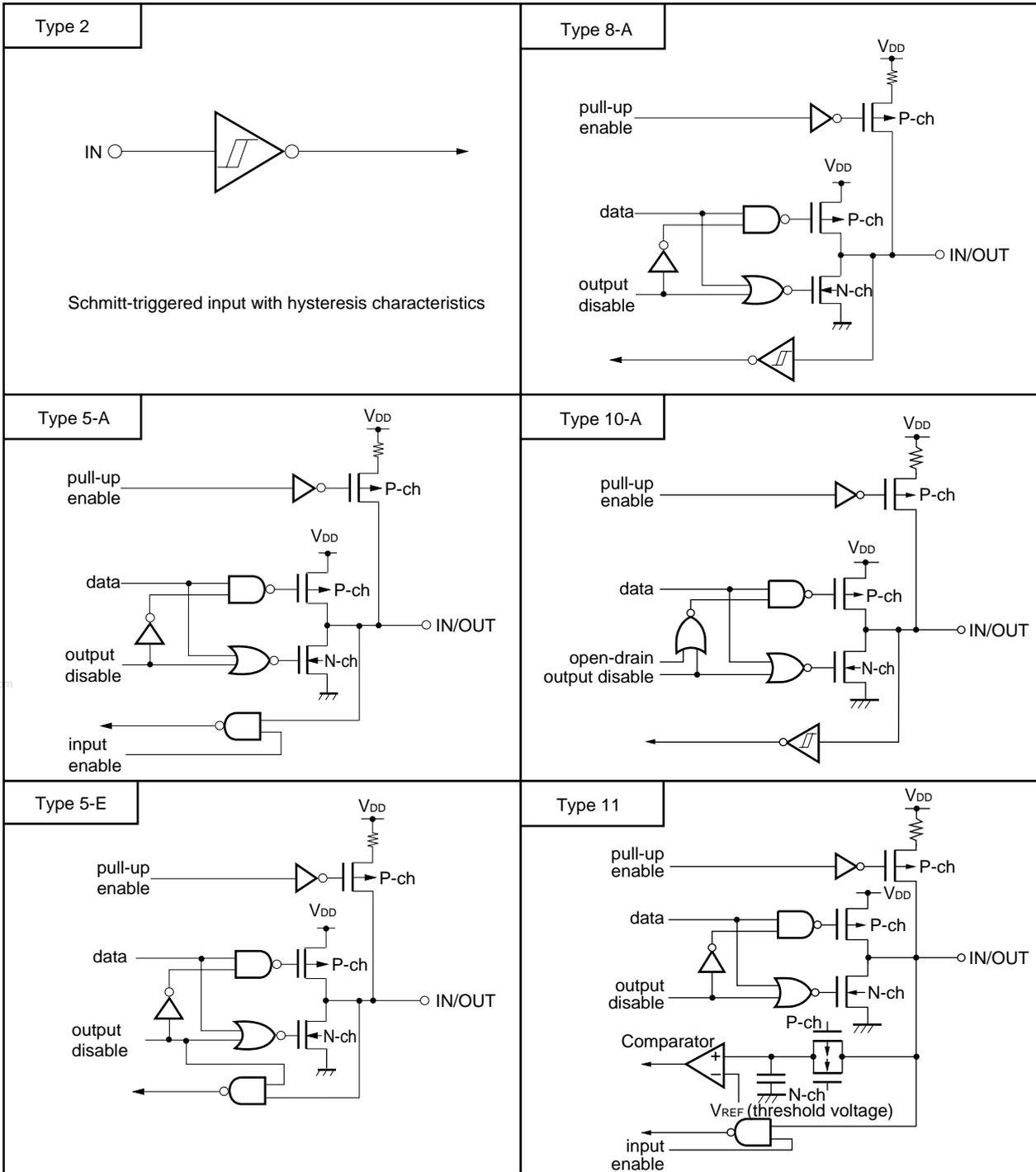
Figure 3-1. Pin Input/Output Circuit List (2/2)
