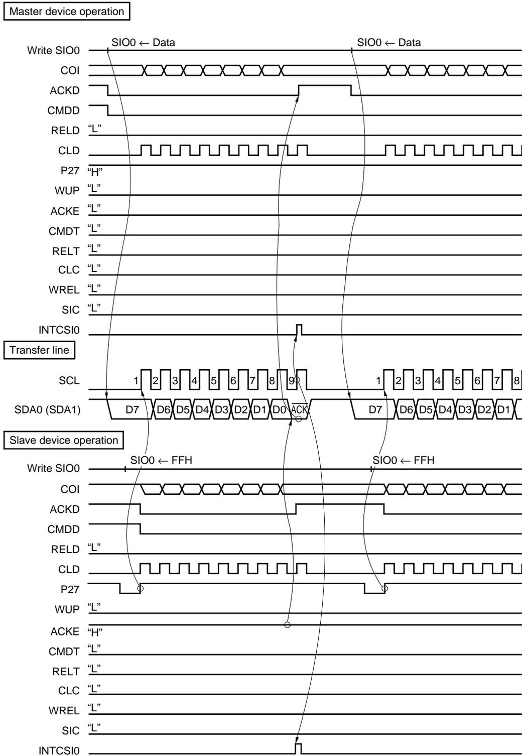
**Figure 16-45. Data Transmission from Master to Slave
