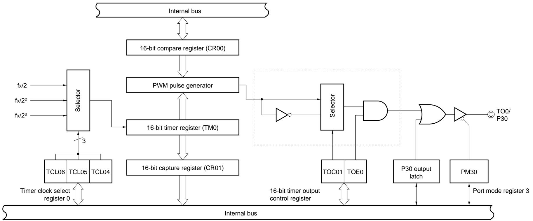
**Remark** The circuitry enclosed by the dotted line is included in the output control circuit.
