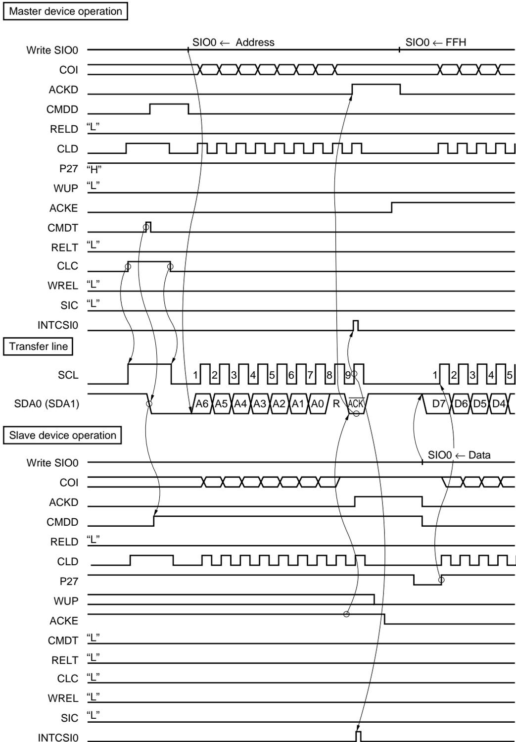
**Figure 16-46. Data Transmission from Slave to Master
