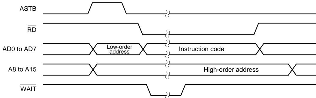
Figure 19-4. External Memory Read Timing
