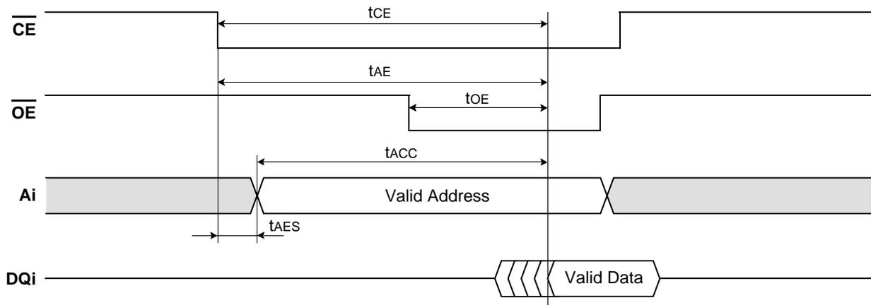
**Latched Asynchronous Read Operation**
