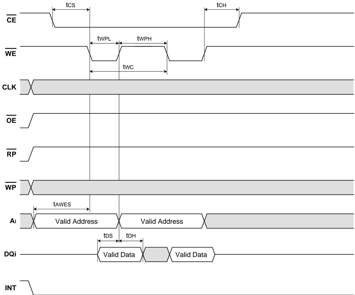
Figure 6. Latched Asynchronous Write Mode
