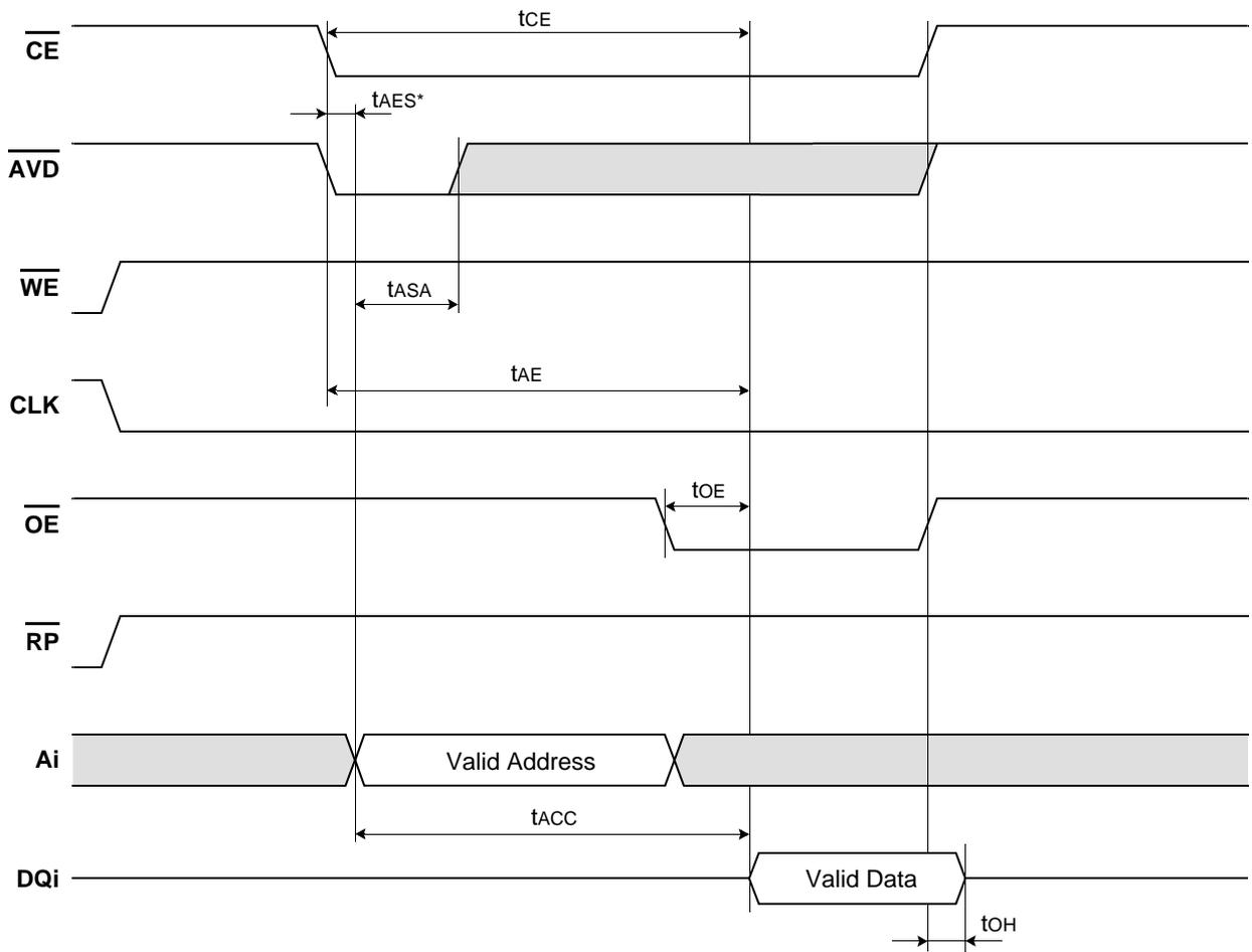
Figure 3. Asynchronous Page Read Mode
