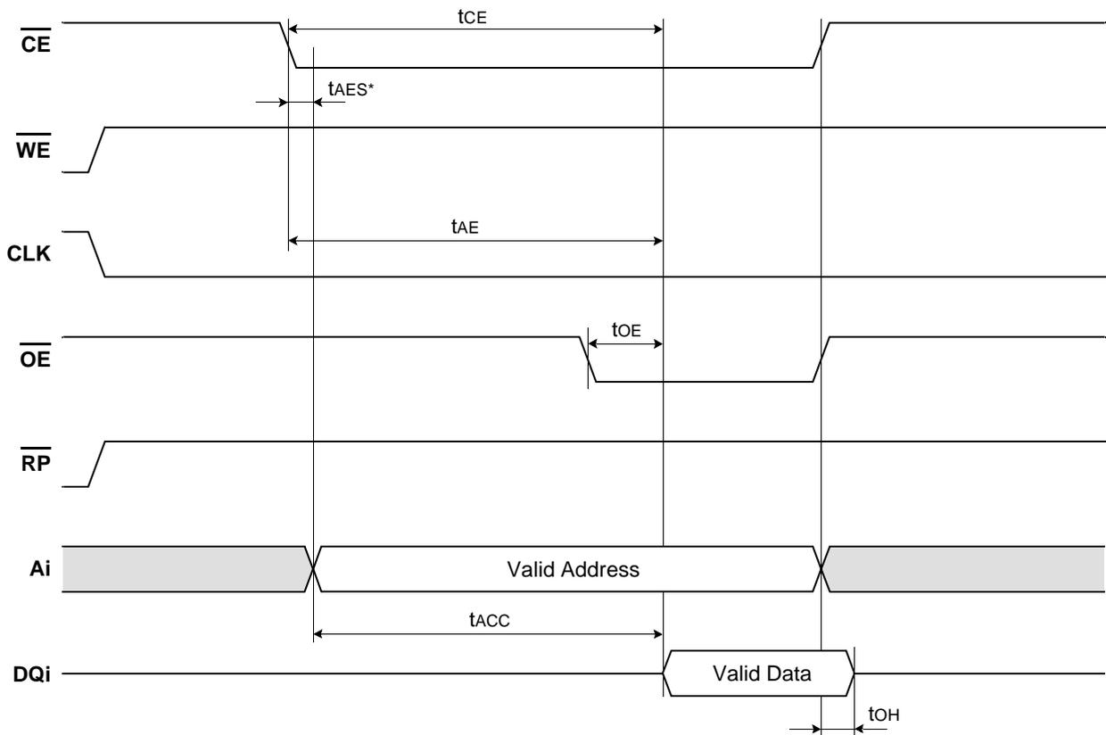
Figure 2. Latched Asynchronous Read Mode
