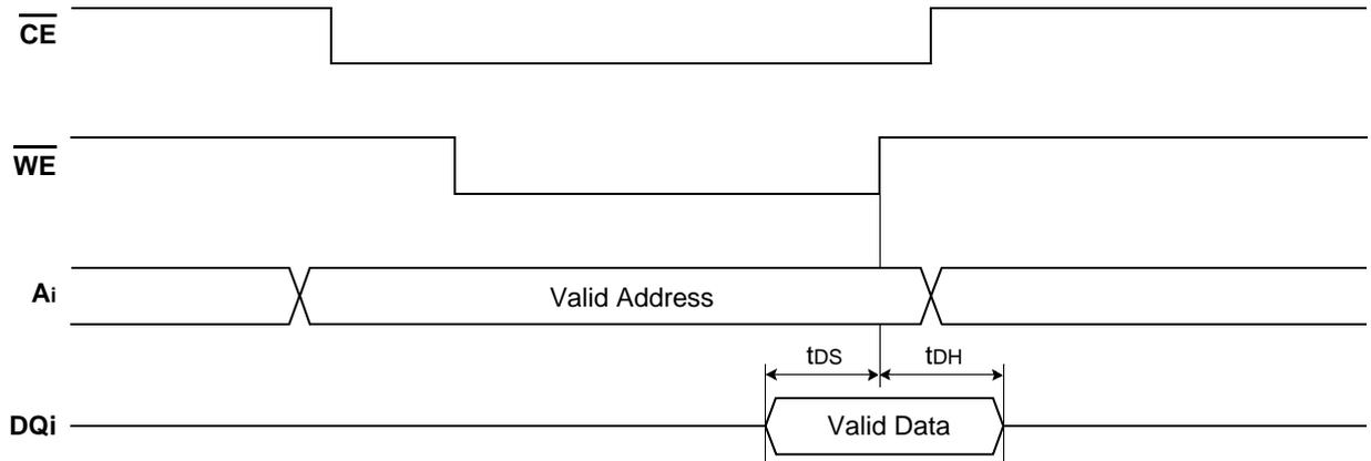
**Latched Asynchronous Write Operation**
