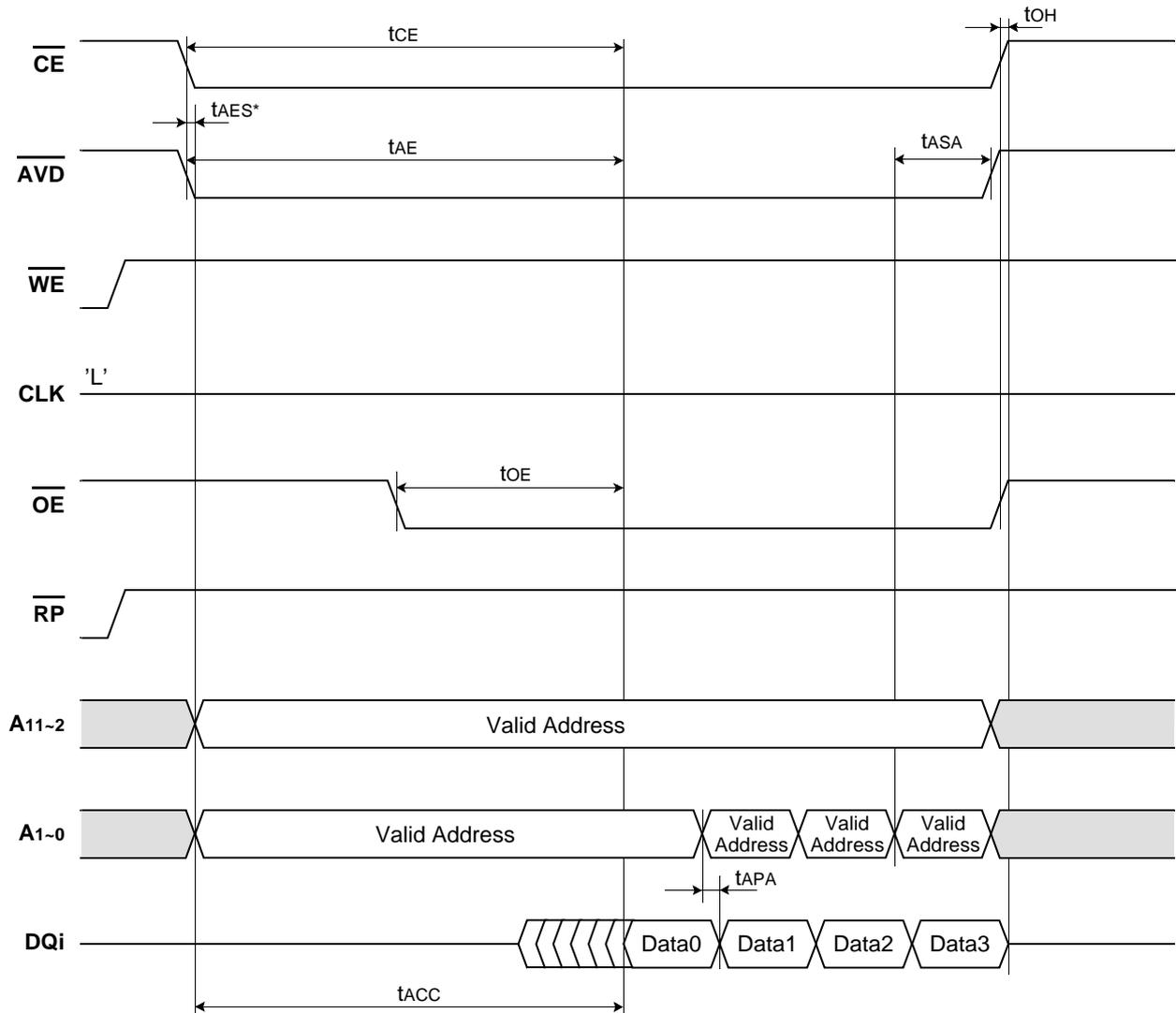
Figure 4. Synchronous Burst Read Mode
