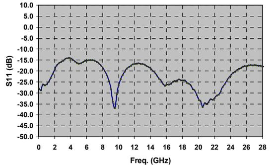
Output Return loss,  $V_{DD}=8V$ ,  $I_{DQ}=220mA$
