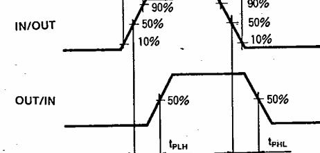
**5 "L-H" and "H-L" output propagation time (CONTROL IN-OUT/IN)**
