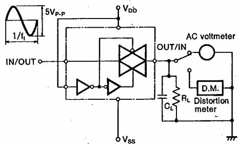
$f_{max}(I/O)$  is taken as that frequency  $f_i$  at which, using a sine-wave input of  $2.5\text{V}_P-P$ ,  $20 \log_{10}(V_O/V_I) = -3\text{dB}$ .
