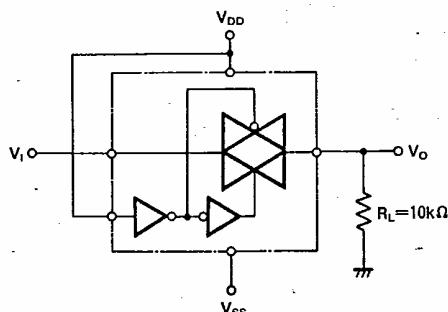
$$R_{ON}=10 \times \frac{(V_I-V_O)}{V_O} \quad (\text{k}\Omega)$$
