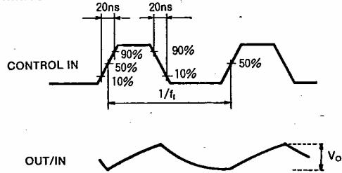
$f_{max}(C_{IN})$  is taken as that frequency  $f_i$  at which the output amplitude ( $V_o$ ) is 1/2 that at 1kHz.
