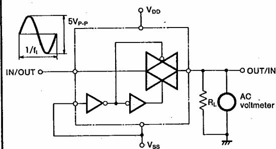
The feedthrough is taken as that frequency  $f_i$  at which, using a sine-wave input of 2.5V\_P-P,  $20 \log_{10}(V_o/V_i) = -50$ dB.
