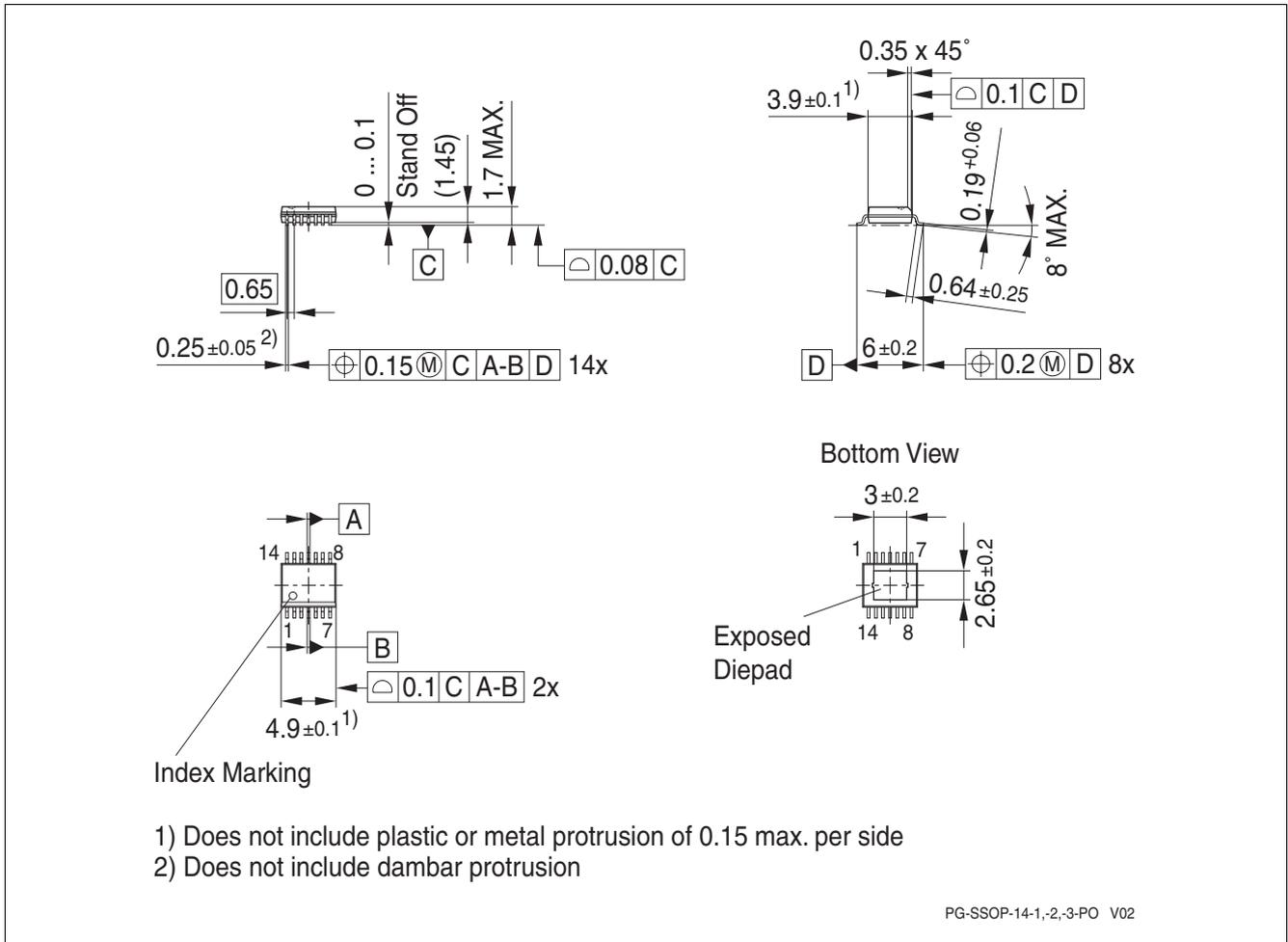
Figure 12 PG-SSOP-14
