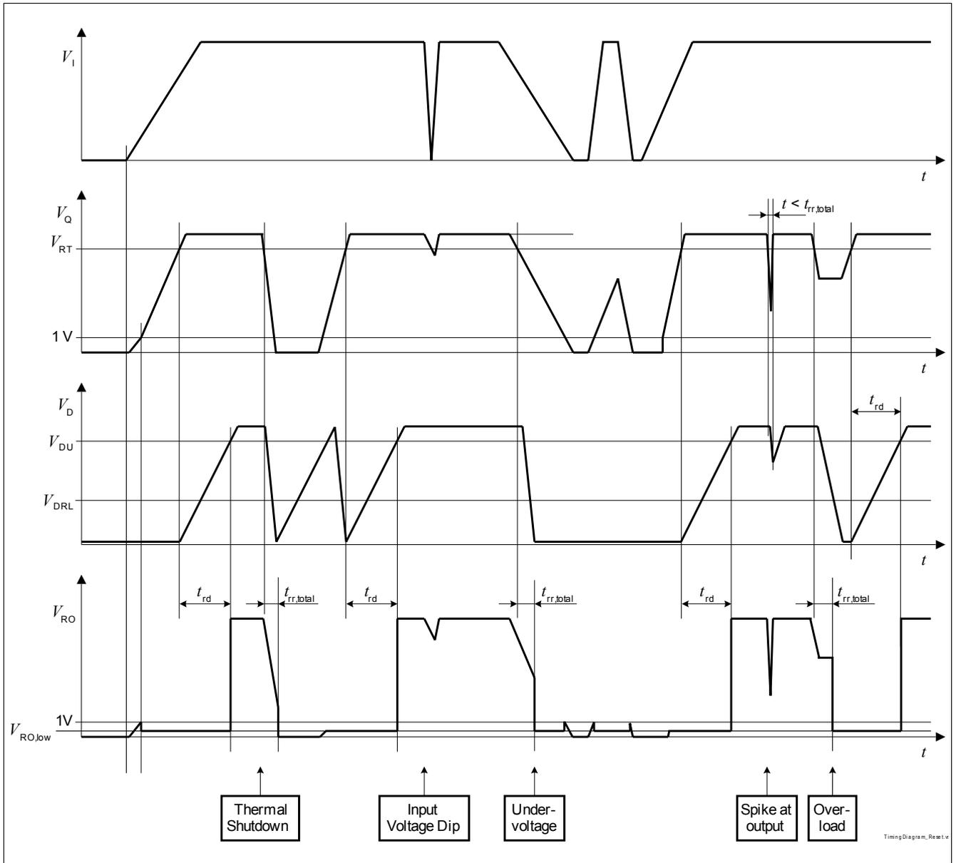
Figure 8 Timing Diagram Reset
