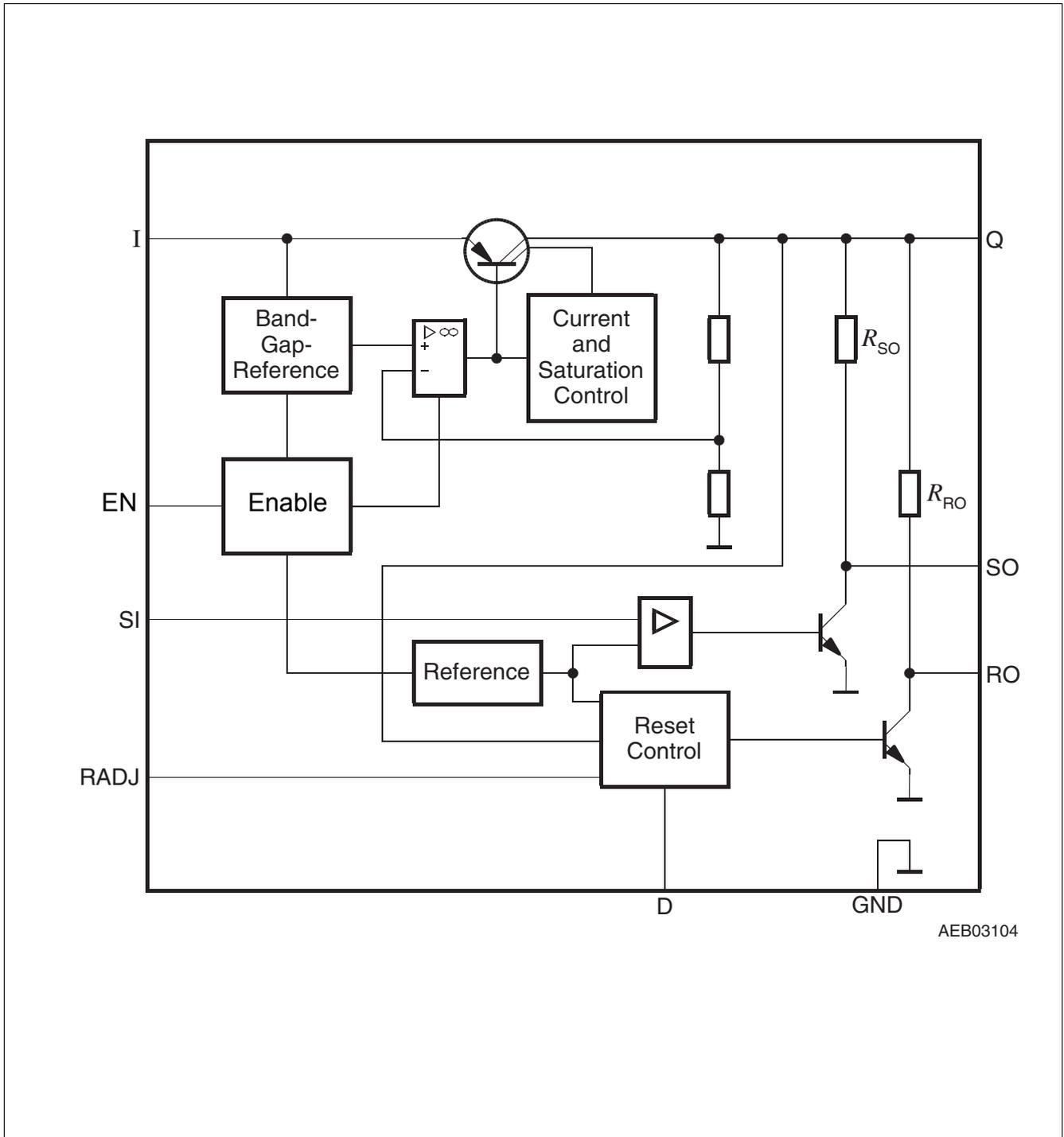
Figure 2 Block Diagram TLE42994GM, TLE42994E (packages PG-DSO-14, PG-SSOP-14)
