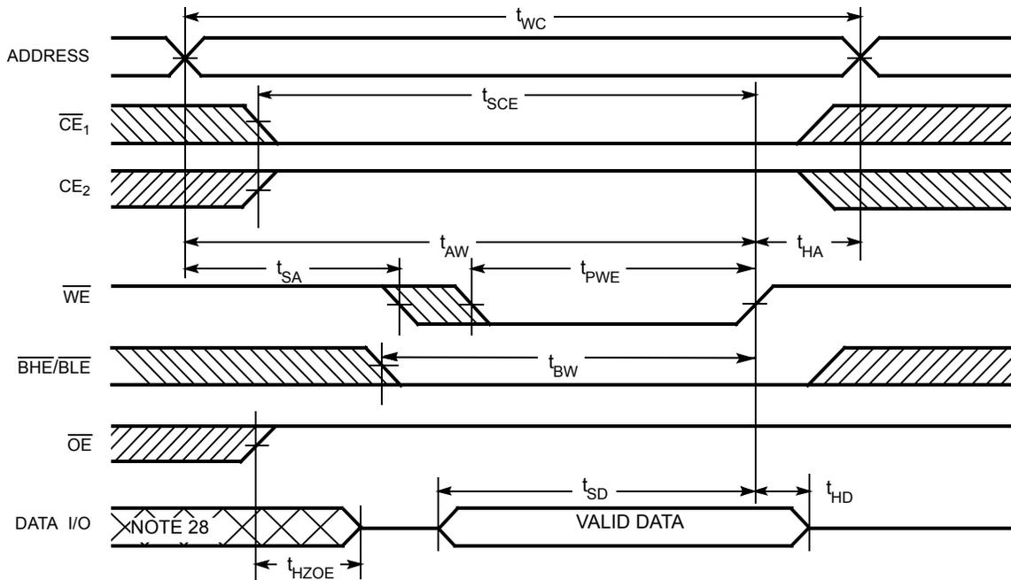
Figure 7. Write Cycle 2 ( $\overline{CE}_1$  or  $\overline{CE}_2$  Controlled) [25, 26, 27, 28]
