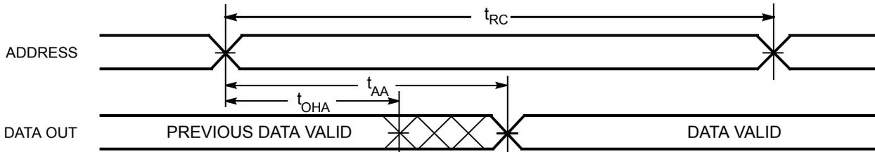
Figure 5. Read Cycle 2 ( $\overline{OE}$  Controlled)<sup>[23, 24]</sup>
