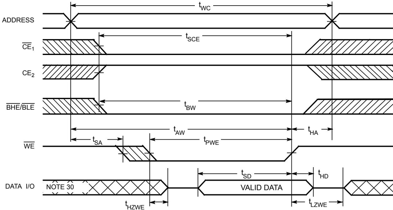
Figure 9. Write Cycle 4 ( $\overline{BHE}/\overline{BLE}$  Controlled,  $\overline{OE}$  LOW)<sup>[29, 30]</sup>
