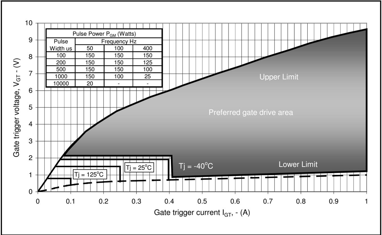
**Fig14 Gate Characteristics**
