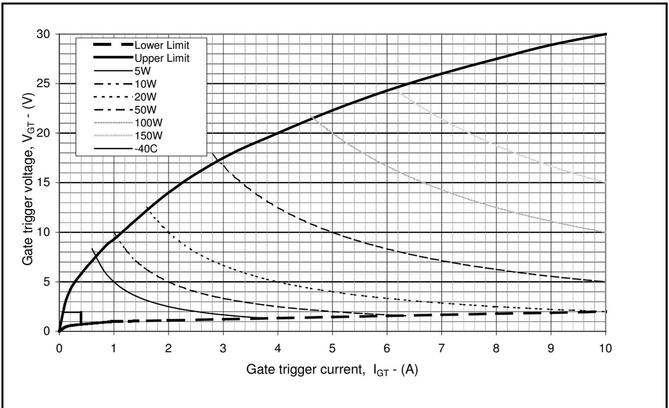
**Fig. 15 Gate characteristics**
