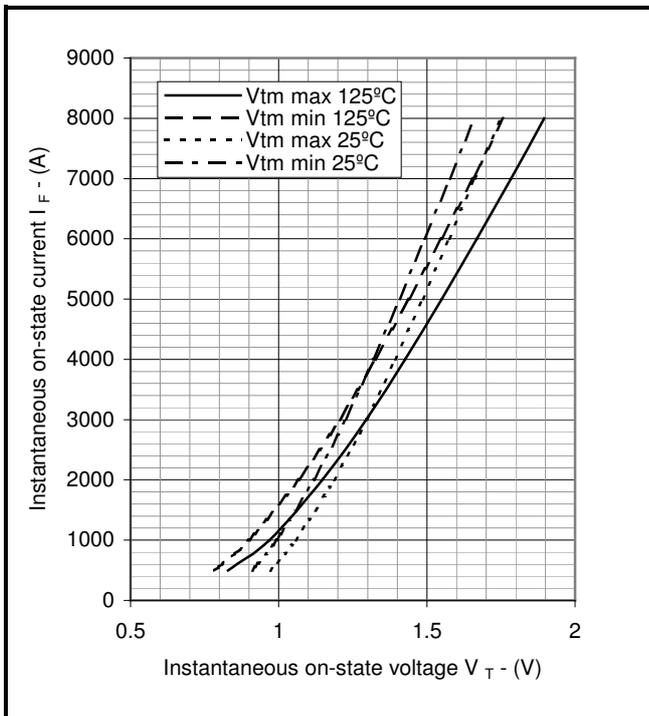
**Fig.2 Maximum & minimum on-state characteristics**
