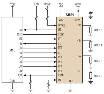
Figure 1. 33894 Simplified Application Diagram
