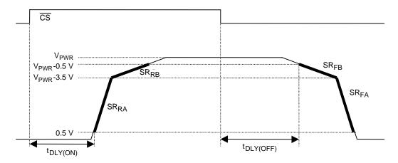
Figure 4. Output Slew Rate and Time Delays
