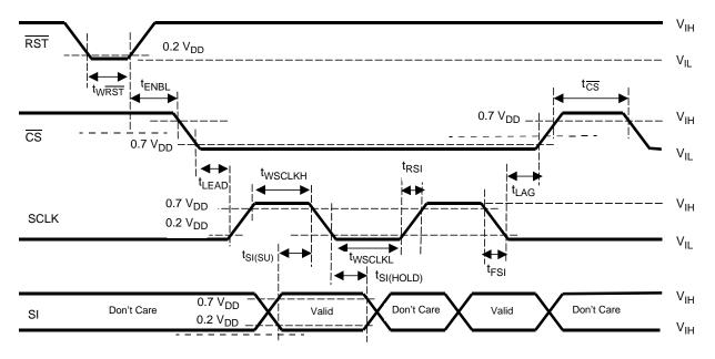
Figure 7. Input timing Switching Characteristics
