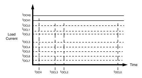
Figure 6. Overcurrent Low and High Detection
