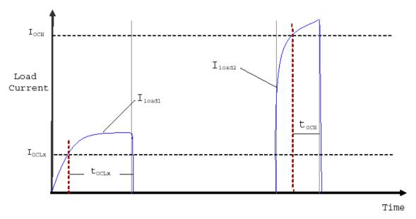
Figure 5. Overcurrent Shutdown
