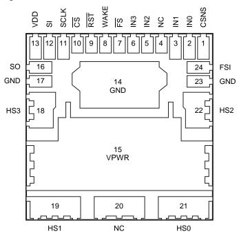
Figure 3. 33894 Pin Connections
