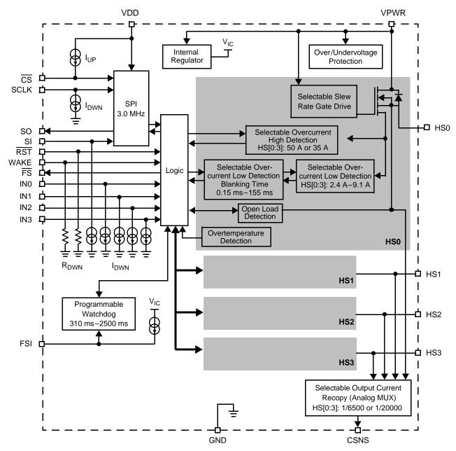
Figure 2. 33894 Simplified Internal Block Diagram
