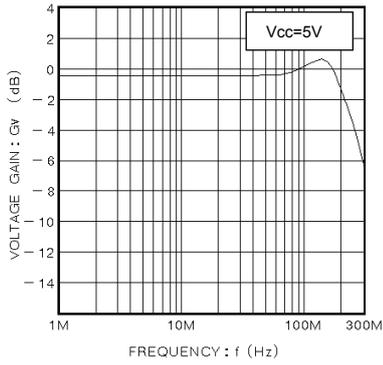
Fig.3 Frequency characteristic
