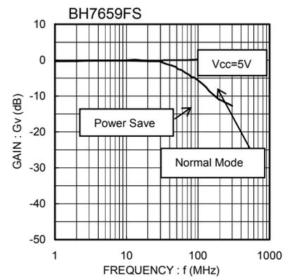
Fig.12 Frequency characteristics
