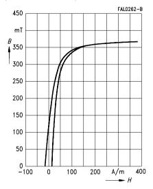
DC magnetic bias (measured on RM cores, typical values)  $(\hat{B} \le 0.25 \text{ mT}, f = 10 \text{ kHz}, T = 25 ^{\circ}\text{C})$
