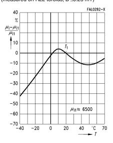
Initial permeability  $\mu_i$  versus temperature (measured on R22 toroids,  $\hat{B} \le 0.25$  mT)
