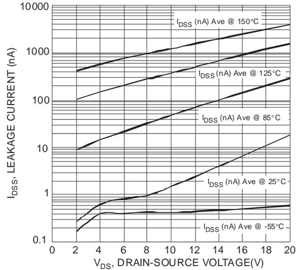
Fig. 10 Typical Drain-Source Leakage Current vs. Voltage
