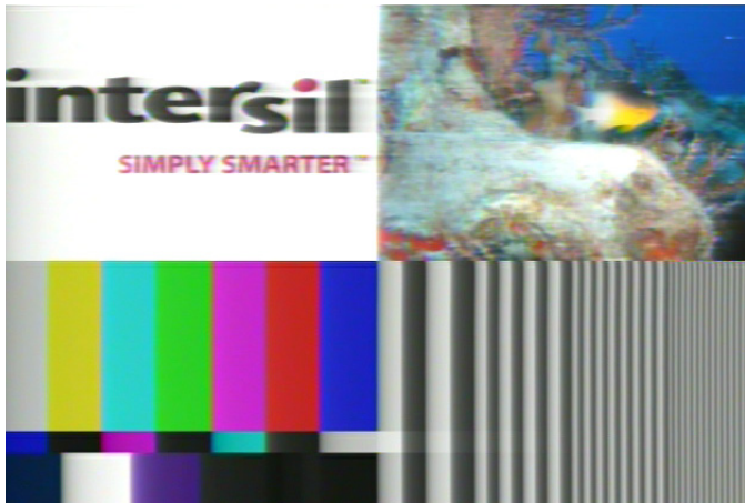
FIGURE 37. TEST PATTERN IMAGE AFTER 5000 FEET OF UNCOMPENSATED RG-59 COAX
