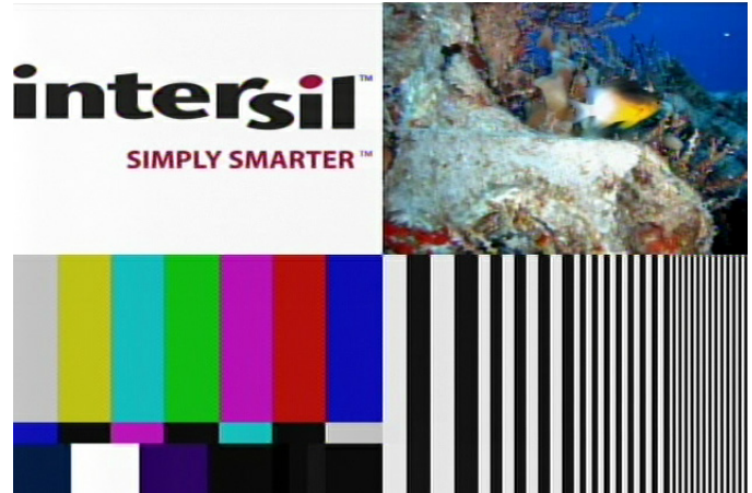
FIGURE 10. TEST PATTERN IMAGE AFTER 3000 FEET OF CAT 5 WITH ISL59603 (OR BETTER)
