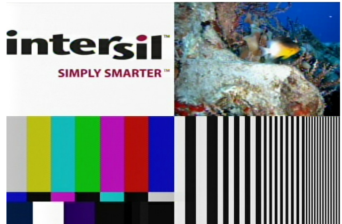
FIGURE 2. TEST PATTERN IMAGE AFTER 1000 FEET OF CAT 5 WITH ISL59601 (OR BETTER)
