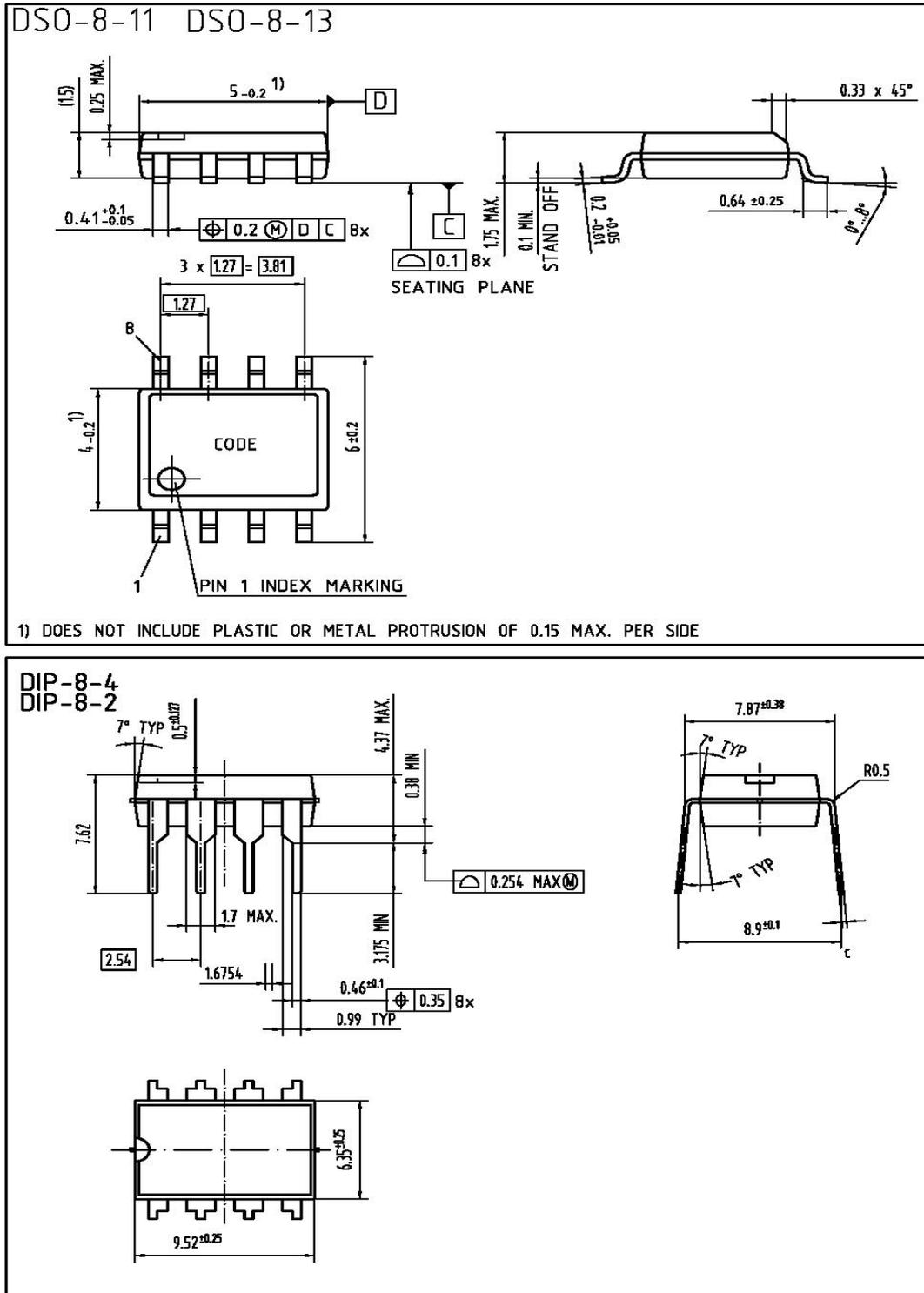
Figure 17 PG-DSO-8 and PG-DIP-8 Outline Dimension
