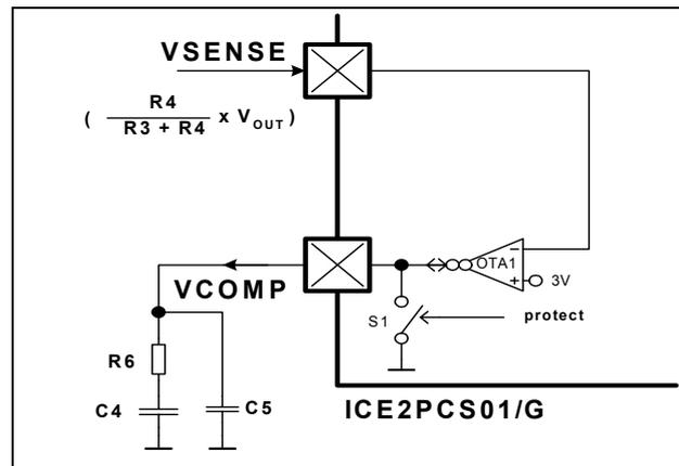
Figure 4 Startup Circuit
